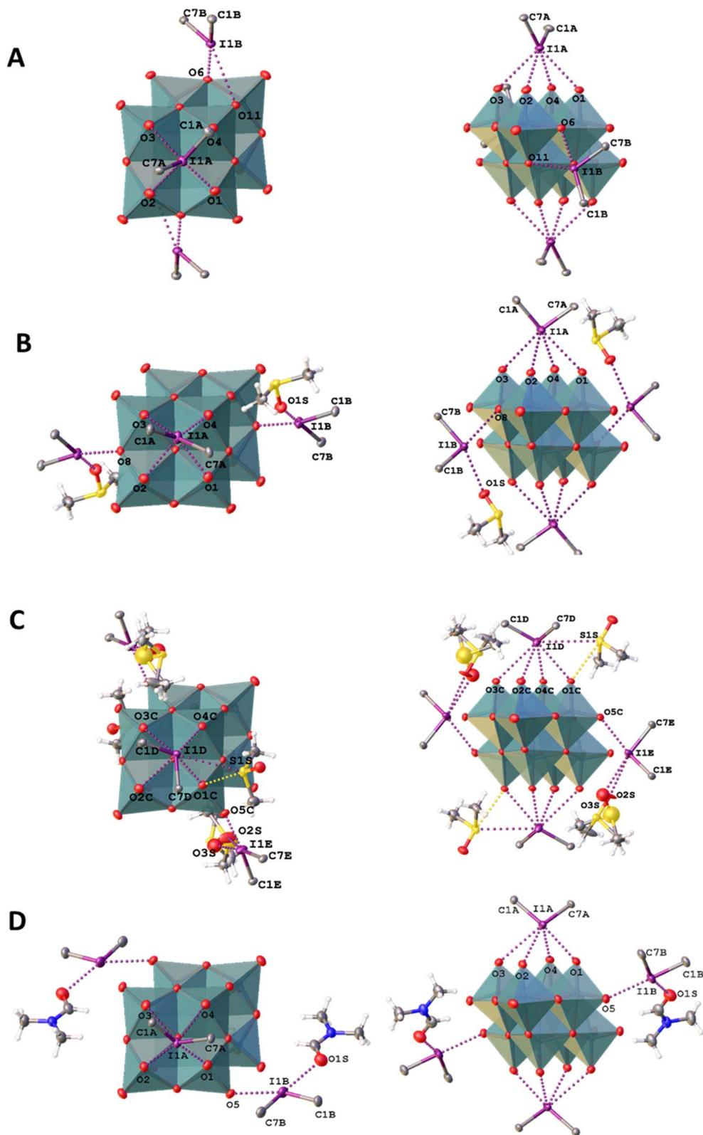
Fig. 2 XB-based linkage patterns of 1–3: (A) 1; (B) 2<sup>I</sup>; (C) 2<sup>II</sup>; (D) 3.
