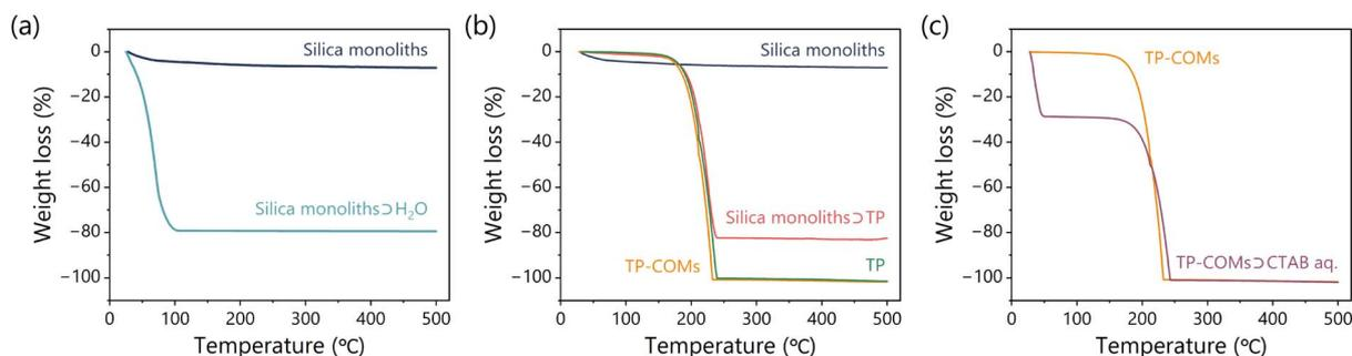
Fig. 2 TGA curves of (a) silica monoliths (black) and silica monoliths exposed to water (blue), (b) silica monoliths (black), composite of silica monoliths and TP (red), TP powder (green), and TP-COMs (orange), (c) TP-COMs (orange) and TP-COMs immersed in the 10 mM aqueous CTAB solution (purple). The same color data represent the same sample.
