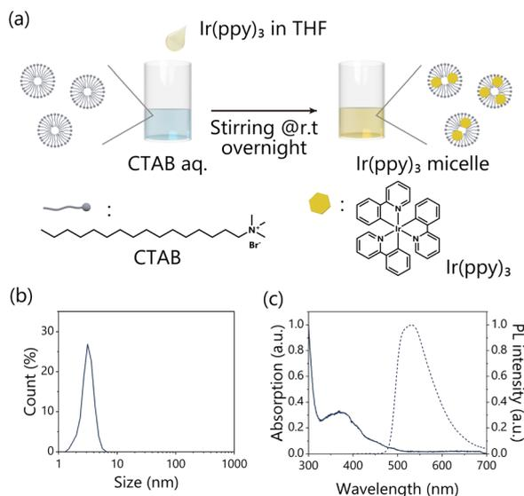
**Fig. 3** (a) Schematic representation of Ir(ppy)<sub>3</sub> micelle preparation and chemical structures of CTAB and Ir(ppy)<sub>3</sub>. (b) DLS profile of Ir(ppy)<sub>3</sub> micelles. (c) UV-vis absorption (solid line) and photoluminescence (dotted line) spectra of Ir(ppy)<sub>3</sub> micelles in water.
