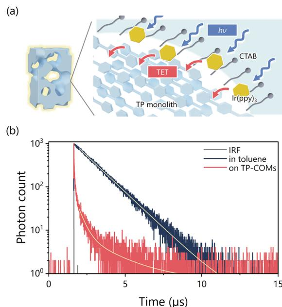
**Fig. 4** (a) Schematic representation of triplet Dexter energy transfer on the macropore surface of TP-COMs. (b) Photoluminescence decays and fitted lines (yellow) of Ir(ppy)<sub>3</sub> in toluene (black) and on the surface of TP-COMs (red). The instrument response function (IRF) is shown in the gray line.
