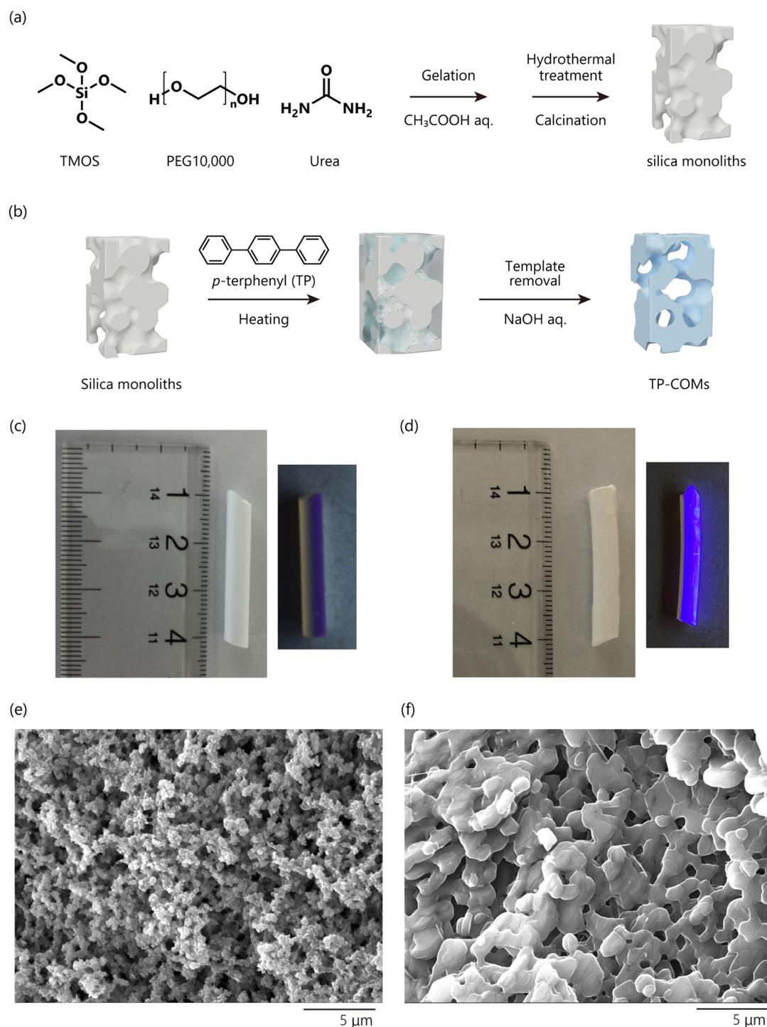
**Fig. 1** (a) Synthetic scheme of silica monoliths. TMOS: tetramethoxysilane and PEG10 000: poly(ethylene glycol) mw: 10 000. (b) Synthetic scheme of TP-COMs. Photographs without (left) and with (right) UV light irradiation of (c) silica monoliths and (d) TP-COMs. (e) SEM images of silica monoliths and (f) TP-COMs.
