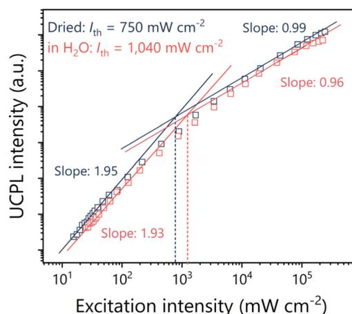
Fig. 6 Excitation intensity dependence of UCPL intensity at 372 nm of Ir(ppy)<sub>3</sub> modified TP-COMs under Ar (black) and in degassed water (red).
