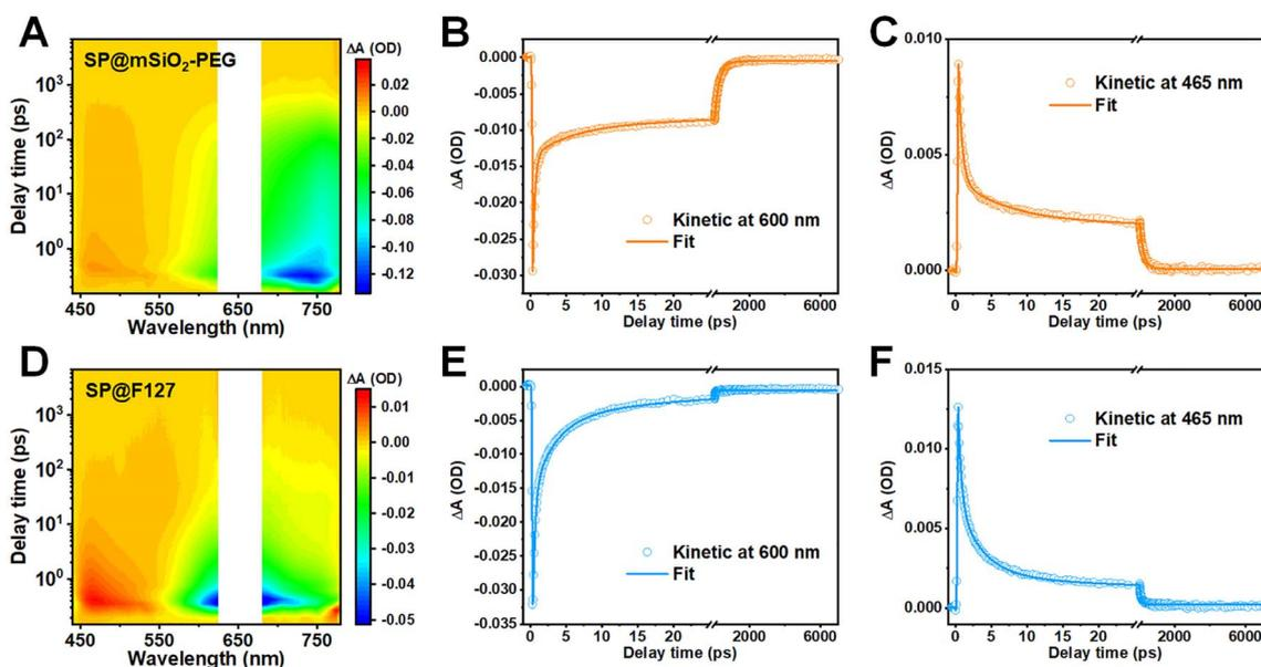
Fig. 3 Investigation of excited state dynamics. 2D pseudocolor fs-TA mapping of (A) SP@mSiO<sub>2</sub>-PEG, and (D) SP@F127 excited with 660 nm laser pulse. Kinetic curves and fitting lines of SP@mSiO<sub>2</sub>-PEG at (B) 600 nm and (C) 465 nm. Kinetic curves and fitting lines of SP@F127 at (E) 600 nm and (F) 465 nm.
