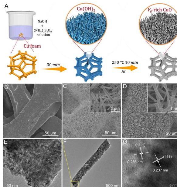
Fig. 1 (A) Schematic illustration of the preparation of the  $\text{V}_\text{o}$ -rich  $\text{CuO}/\text{CF}$  electrode. (B) SEM image of bare Cu foam. (C) SEM image ((inset): enlargement) of  $\text{Cu}(\text{OH})_2$  arrays grown on Cu foam. The inset shows the enlarged  $\text{Cu}(\text{OH})_2$  nanorods. (D) SEM image ((inset): enlargement) of  $\text{V}_\text{o}$ -rich CuO on Cu foam. (E and F) TEM images and (G) HRTEM image of a single  $\text{V}_\text{o}$ -rich CuO nanorod.
