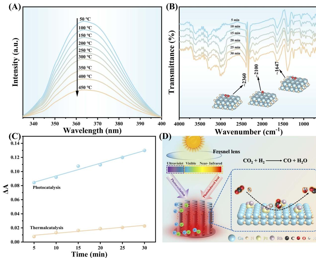
Fig. 3 (A) TD-PL spectroscopy of PtRh/GaN NWs/Si. (B) *Operando* DRIFT spectra of CO<sub>2</sub> hydrogenation over PtRh/GaN NWs/Si under light illumination of 4.3 W cm<sup>-2</sup>. Ga, blue; N, orange; C, gray; O, red; and H, white. (C) Slope change of the peak intensity of \*COOH calculated based on (B) and Fig. S17.† (D) Schematic diagram of the synergy effect of photothermal synergistic for promoting CO<sub>2</sub> hydrogenation over PtRh/GaN NWs/Si.
