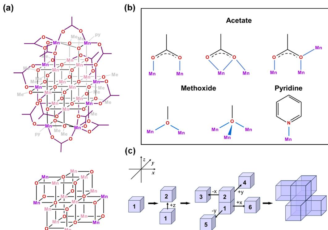
Fig. 2 (a) Schematic illustrations of the  $[\text{Mn}_{18}\text{-Ac}]$  cluster and its  $[\text{Mn}_4\text{O}_4]$ -assembled core. Pink and purple colors designate  $\text{Mn}^{\text{III}}$  and  $\text{Mn}^{\text{II}}$  ions, respectively. (b) The coordination modes of acetate, methoxide, and pyridine in  $[\text{Mn}_{18}\text{-Ac}]$ . (c) Schematic representation of the assembling  $[\text{Mn}_4\text{O}_4]$  cubic units in the core structure of  $[\text{Mn}_{18}\text{-Ac}]$ .
