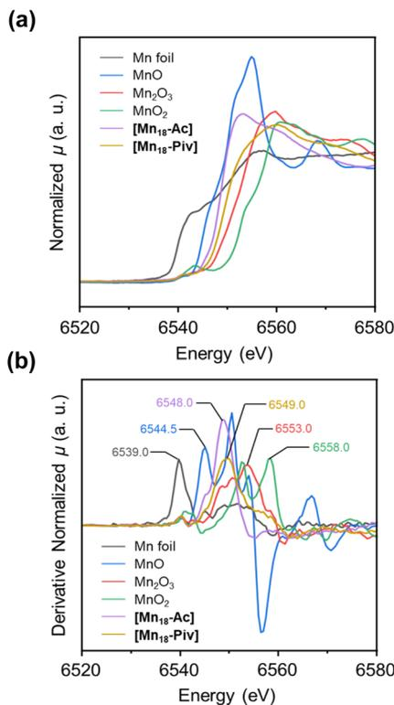
Fig. 5 Normalized XANES spectra (a) and the first-derivative normalized XANES spectra (b) for Mn<sup>0</sup> foil, Mn<sup>II</sup>O, Mn<sup>III</sup><sub>2</sub>O<sub>3</sub>, Mn<sup>IV</sup>O<sub>2</sub>, [Mn<sub>18</sub>-Ac], and [Mn<sub>18</sub>-Piv].
