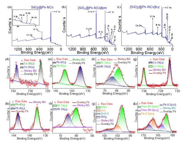
Fig. 2 XPS survey plots of (a)  $SiO_2@Pv-NCs$ , (b)  $[SiO_2@Pv-NCs]tpm$ , and (c)  $[SiO_2@Pv-NCs]tsy$ . High-resolution X-ray photoelectron spectra for Pv-NCs: (d) Cs (3d), (e) Pb (4f), (f) Br (3d), (g) Cs (3d); and for  $SiO_2@Pv-NCs$  (h) Pb (4f), (i) Br (3d), (j) Si (2p), and (k) S (2p) regions.
