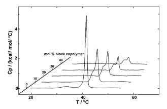
Fig. 3 DSC experiments showing the endotherms of HVs made of DPPC with increasing PMOXA21-b-PDMS $_{73}$ -b-PMOXA $_{21}$  content. Reprinted with permission from ref. 1. Copyright 2024 American Chemical Society.
