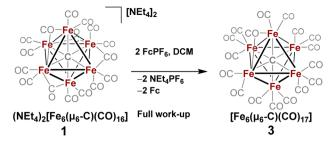
Scheme 3 In situ oxidation of 1 in non-coordinating solvent to form 3, the stable six-iron close cluster
