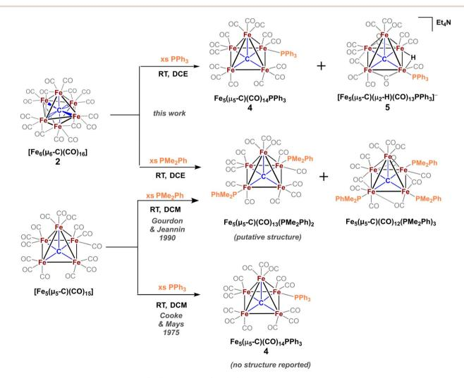
Scheme 4 Reactions of the neutral, six-iron (top) and five-iron (bottom) clusters with the monodentate phosphines  $PMe_2Ph$  and  $PPh_3$  to form singly, doubly, and triply bound phosphine supported five-iron clusters.
