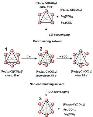
Scheme 1 Oxidation of 1 (center left) to form the key hypercloso intermediate 2, (center). The subsequent reaction with the CO atmosphere forms an intact and isolable *nido* cluster (center right). Without CO, it forms the two disproportionate families of iron(carbide) carbonyls shown at top and bottom in coordinating and non-coordinating solvents, respectively. The intact and isolable cluster 3 is only formed and stable in non-coordinating solvent, unlike all the other clusters shown.
