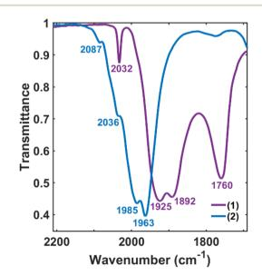
Fig. 1  $\,$  IR spectra of drop-cast samples during the oxidation of 1 (violet) to form 2 (blue) in MeCN.
