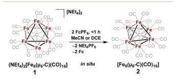
Scheme 2 In situ oxidation of 1 to form the non-PSEPT intermediate 2, the key precursor to all of the ligand additions in this report.
