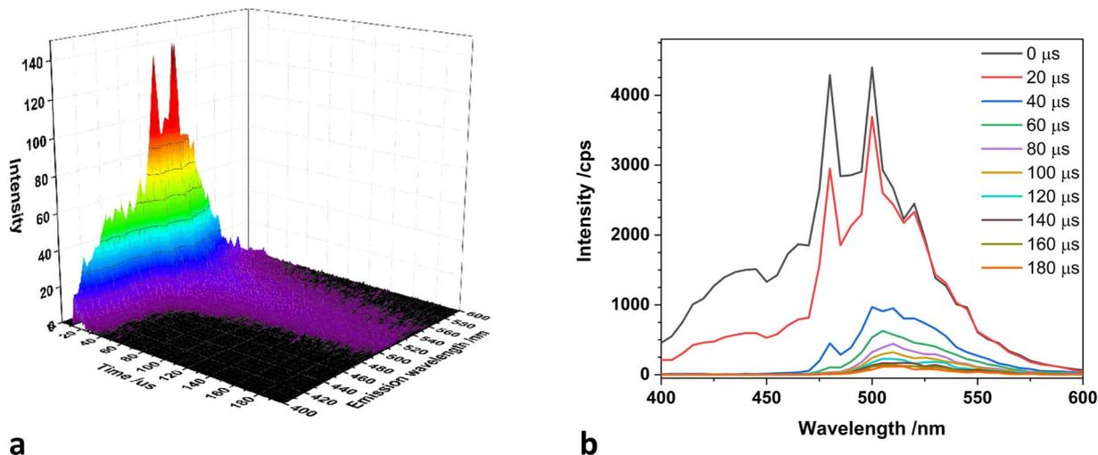
Fig. 4 (a) Time resolved emission spectra map and (b) spectra recorded with increasing time delay (B) of  $1\text{-NO}_3$  in MeCN at room temperature.
