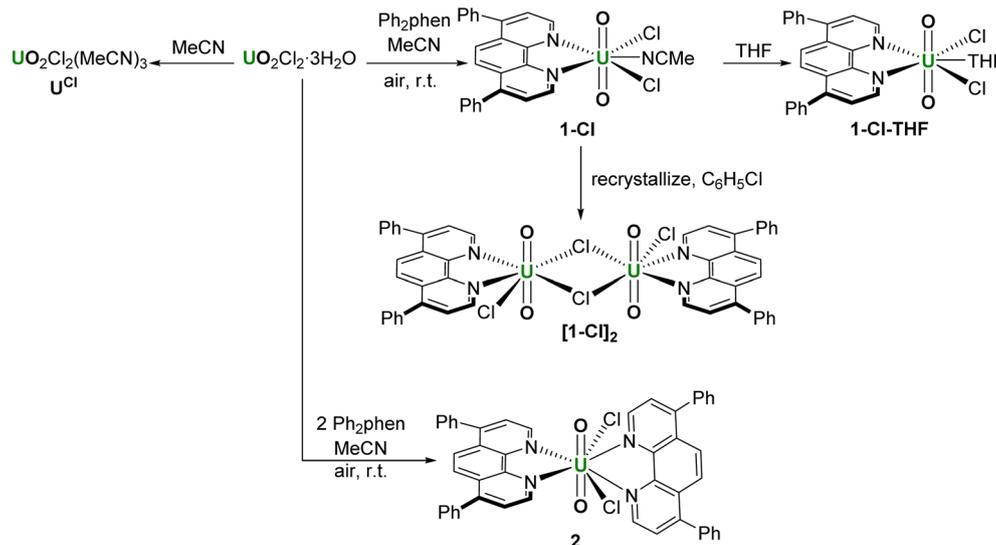
Scheme 1 The uranyl chloride complexes made for comparison with 1-NO<sub>3</sub>, containing 0, 1, and 2 Ph<sub>2</sub>phen ligands.
