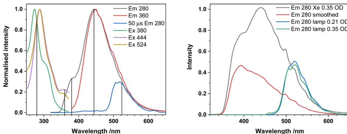
Fig. 5 Left; Absorption, emission, and excitation spectra of **2** dissolved in MeCN (present as **1-Cl** +  $\text{Ph}_2\text{phen}$ ) at room temperature. The blue trace was recorded using a 50 microsecond time delay and gate and shows the longer-lived uranyl emission can be resolved after the shorter lived emission centred at 380 and 444 nm has decayed.
