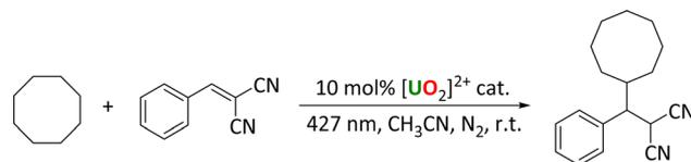
Scheme 3 Photocatalytic cyclooctane addition to benzylidene malononitrile.
