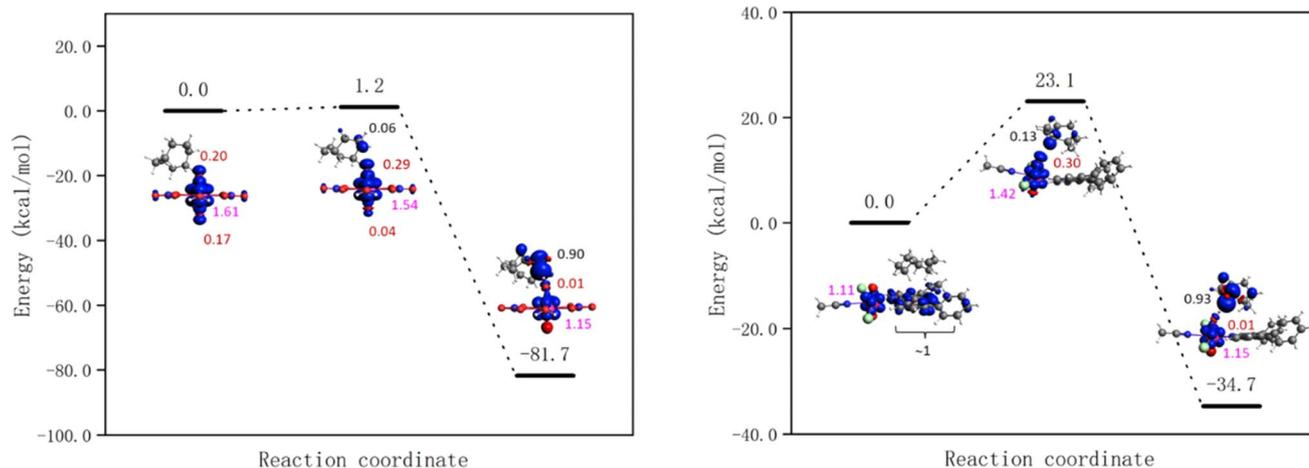
Fig. 9 Energy profiles for HAT from cyclooctane by the excited state of  $[\text{UO}_2(\text{NO}_3)_2(\text{H}_2\text{O})_2]$   $\text{U}^{\text{NO}_3}$  (left) and  $[\text{UO}_2\text{Cl}_2(\text{Ph}_2\text{phen})(\text{MeCN})]$  **1-Cl** (right) calculated at the DLPNO-CCSD(T)//scalar-ZORA PBE0-D3BJ/TZP level of theory. Spin density of reactant, transition state, and product are shown (spins on different atoms are marked in different colours: Cl – azure, O – red, U – pink, and C – black).
