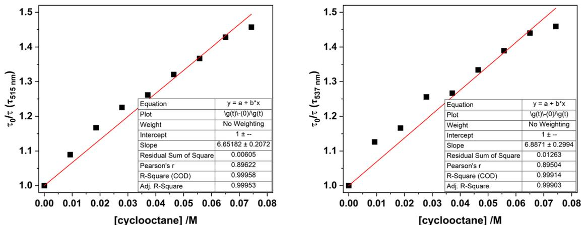
Fig. 14 Stern–Volmer plots for samples of 1-Cl in MeCN, comparing the luminescence lifetimes ( $\lambda_{\text{ex}} = 427$  nm) monitored at 515 nm (left) and 537 nm (right) with increasing amounts of cyclooctane.
