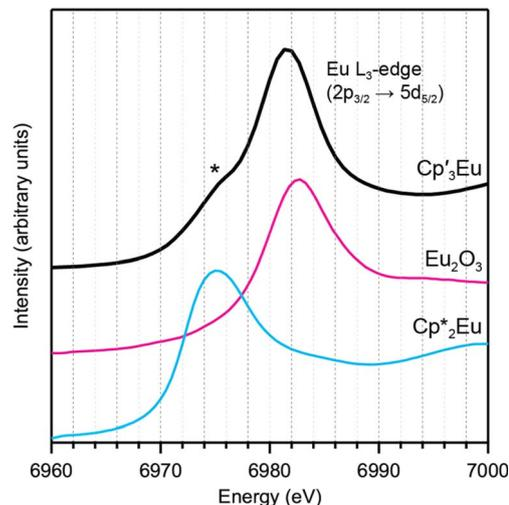
Fig. 4  $L_3$ -edge spectrum for  $Cp'_3Eu$  (magenta) and references for  $Eu^{3+}$  ( $Eu_2O_3$ , dashed black) and  $Eu^{2+}$  ( $Cp_2^*Eu$ , dashed blue). A curve fit of the experimental data for  $Cp'_3Eu$  is provided in the ESI† (Fig. S12†). A shoulder associated with  $Eu^{2+}$  character in the  $L_3$ -edge spectrum for  $Cp'_3Eu$  is highlighted with an asterisk.
