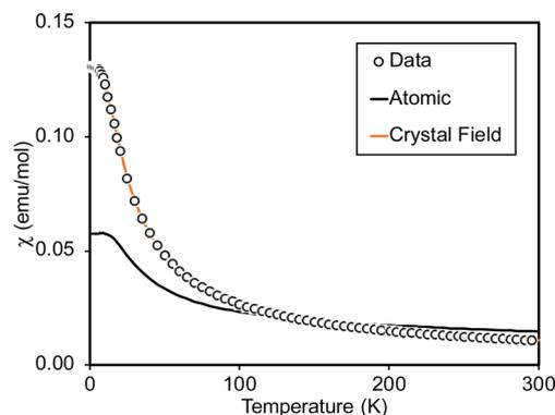
Fig. 5 Magnetic susceptibility of  $Cp'_3Eu$  (open circles). The fit using eqn (4) (free-ion model) is shown as a solid black line. The results of fitting the data using CONDON 3 (crystal field model with  $k = 0.7$ ) is shown using an orange line.
