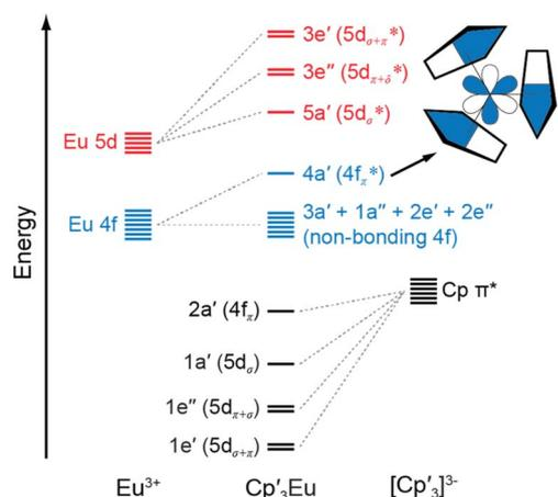
Fig. 1 A qualitative MO diagram of Cp<sub>3</sub>Eu in C<sub>3h</sub> symmetry. The inset shows the a' antibonding interaction of metal f and ligand orbitals. The nodal characteristics of the (Cp<sub>3</sub>)<sup>3-</sup> fragment relative to the metal atom are represented with common short-hand notation.<sup>53,57</sup>
