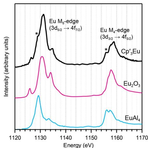
Fig. 3  $M_{5,4}$ -edge spectrum for  $\text{Cp}'_3\text{Eu}$  (black) and references for  $\text{Eu}^{3+}$  ( $\text{Eu}_2\text{O}_3$ , magenta) and  $\text{Eu}^{2+}$  ( $\text{EuAl}_4$ , blue). Two features associated with  $\text{Eu}^{2+}$  character in the  $L_{3-}$ -edge spectrum for  $\text{Cp}'_3\text{Eu}$  are highlighted with asterisks.
