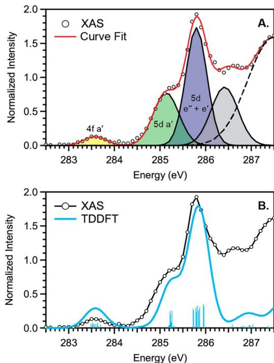
Fig. 2 (A) C K-edge XAS pre-edge of  $\text{Cp}'_3\text{Eu}$  (black circles), Gaussian functions (yellow, green, blue, and gray), and the sum of post-edge functions (dashed black trace) used to generate the total curve fit (red). (B) C K-edge XAS experimental data for  $\text{Cp}'_3\text{Eu}$  (black circles), the TDDFT-calculated spectrum (blue) and calculated transitions (vertical blue bars). The three main features are labeled with the acceptor MOs from the transition assignments.
