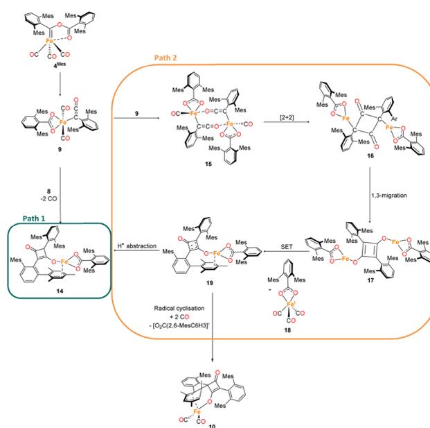
Scheme 4 Two potential routes to **14** via proposed complex **9**. Path 1 forms **14** via a [2 + 2] cycloaddition of **8** and **9**. Path 2 forms **14** through dimerization of **9** then a [2 + 2] cyclisation, followed by 1,3 migration and a single electron transfer, giving **18** and **19**. Path 2 also has the potential to form decomposition complex **10** via radical cyclisation of **19**.
