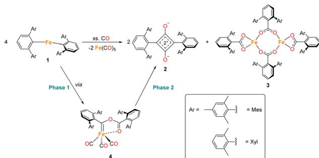
**Scheme 1** General reaction scheme for the reaction between **1** in the presence of CO, where Ar = Mes or Xyl. The two phases of the reaction are shown, phase 1 covers the reaction of **1** to **4**, phase 2 covers the reaction from **4** to **2**, **3** and  $\text{Fe}(\text{CO})_5$ .
