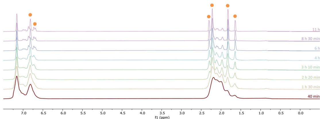
Fig. 2  $^1\text{H}$  NMR spectra (–1 to 8 ppm) of the reaction between CO and  $1^{\text{Mes}}$  ( $\text{C}_6\text{D}_6$ , 1 atm CO, room temperature) recorded between 40 minutes and 11 hours of reaction. Orange circles highlight the signals for  $4^{\text{Mes}}$ .
