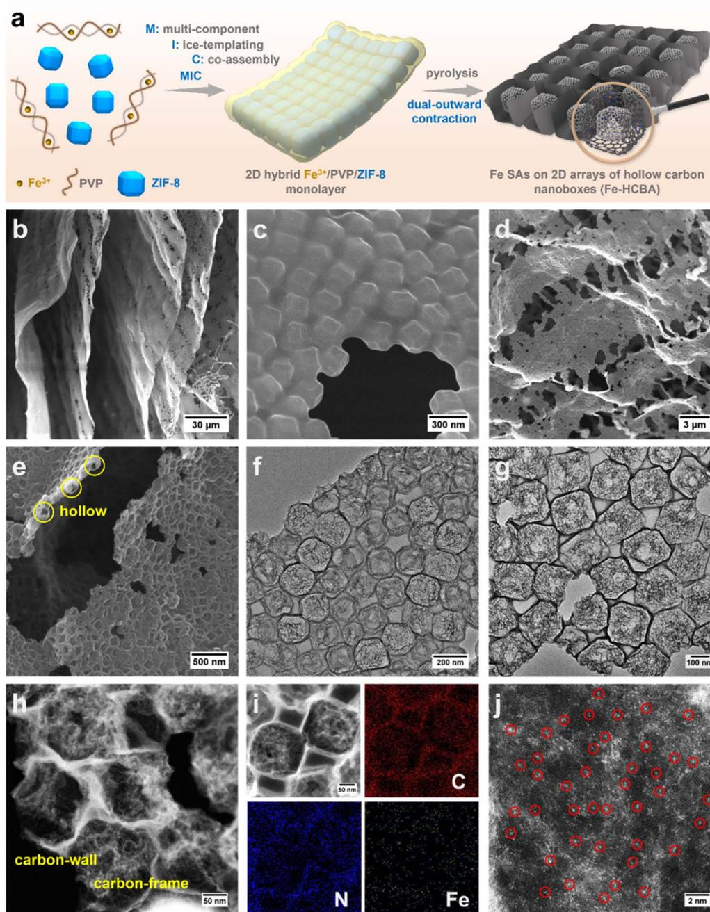
Fig. 1 (a) Schematic illustration of the synthetic process for Fe-HCBA. (b and c) SEM images of Fe<sup>3+</sup>/PVP/ZIF-8-2. (d and e) SEM, (f and g) TEM, (h and i) Scanning TEM (STEM) images and the corresponding elemental mapping of Fe-HCBA-2, and (j) atomic-resolution HAADF-STEM of Fe-HCBA-2.
