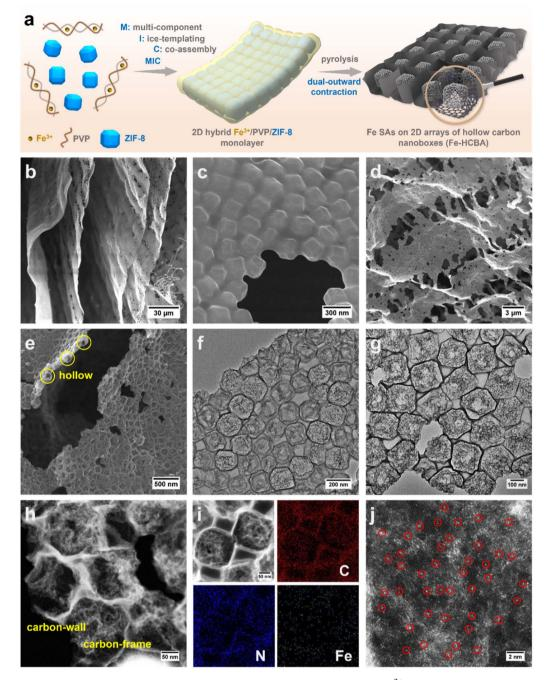
Fig. 1 (a) Schematic illustration of the synthetic process for Fe-HCBA. (b and c) SEM images of  $Fe^{3+}/PVP/ZIF-8-2$ . (d and e) SEM, (f and g) TEM, (h and i) Scanning TEM (STEM) images and the corresponding elemental mapping of Fe-HCBA-2, and (j) atomic-resolution HAADF-STEM of Fe-HCBA-2.
