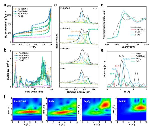
Fig. 3 (a)  $N_2$  sorption isotherms, (b) NLDFT pore size distribution plots, and (c) N 1s XPS spectra of Fe-HCBA-1, Fe-HCBA-2, Fe-HCBA-3 and Fe-NC. (d) Fe K-edge XANES spectra, (e) FT  $k^2$ -weighted Fe K-edge EXAFS spectra, and (f) 3D contour WT-EXAFS plots of Fe-HCBA-2 and reference samples.
