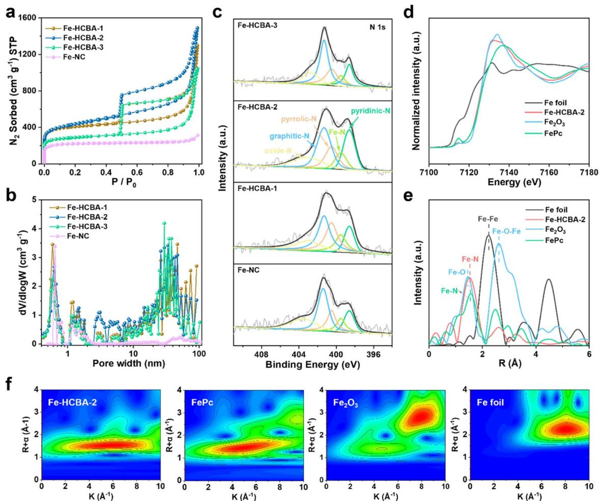
Fig. 3 (a)  $N_2$  sorption isotherms, (b) NLDFT pore size distribution plots, and (c) N 1s XPS spectra of Fe-HCBA-1, Fe-HCBA-2, Fe-HCBA-3 and Fe-NC. (d) Fe K-edge XANES spectra, (e) FT  $k^2$ -weighted Fe K-edge EXAFS spectra, and (f) 3D contour WT-EXAFS plots of Fe-HCBA-2 and reference samples.
