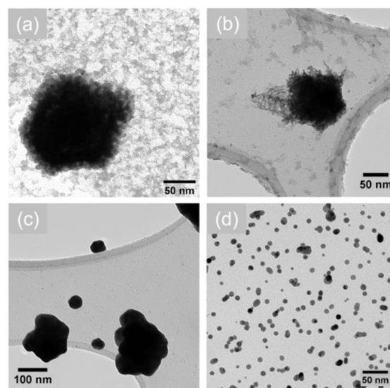
Fig. 3 TEM images of AuNPs produced from (a) control treatment with 34.3 mM H<sub>2</sub>O<sub>2</sub>, (b) afterglow treatment in He/Ar at 6 W, (c) afterglow treatment in He/Ar/H<sub>2</sub>O at 14 W, and (d) plasma-treated gold precursor droplet in He/Ar/H<sub>2</sub>O at 14 W.
