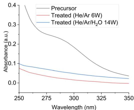
Fig. 2 The averaged UV-vis absorbance profiles of precursor and solutions treated by He/Ar plasma at 6 W and He/Ar/H<sub>2</sub>O plasmas at 12 W at a total gas flow rate of 2 slm. All the solutions were diluted 10 times.
