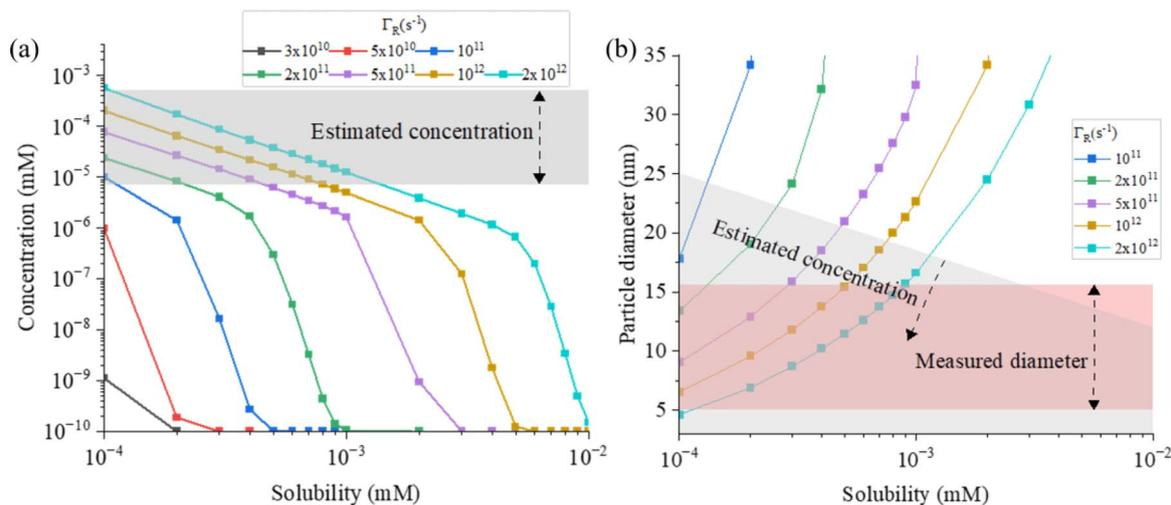
Fig. 5 The (a) concentration and (b) diameter plots of AuNPs from simulations where reducing flux was varied from  $3 \times 10^{10} \text{ s}^{-1}$  to  $2 \times 10^{12} \text{ s}^{-1}$  (diffusion-limited) and the solubility of gold monomers was varied from  $10^{-4}$  to  $10^{-2}$  mM. From the experiment with He/Ar/ $\text{H}_2\text{O}$  plasma, the concentration and diameter lie between  $7 \times 10^{-6}$ – $5 \times 10^{-4}$  mM and 5.0–14.5 nm, respectively.
