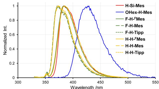
Fig. 3 PL spectra of benzo[d]dithieno[b,f]borepins in THF at room temperature.
