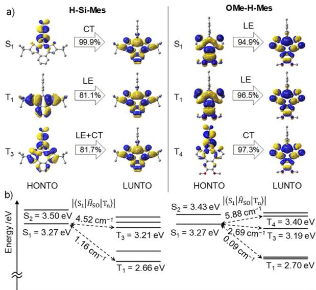
Fig. 7 (a) NTOs of H-Si-Mes and OMe-H-Mes in the S<sub>0</sub> geometry at the B3LYP/6-31G(d) level of theory. (b) Calculated singlet and triplet energy levels and SOCMEs at the B3LYP/6-31G(d) level of theory.
