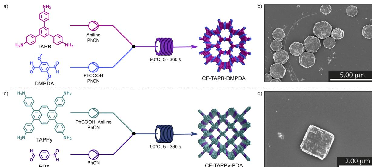
Fig. 1 Continuous flow synthesis of single-crystalline **CF-TAPB-DMPDA** (a) and **CF-TAPPy-PDA** (c) covalent organic frameworks. Scanning electron microscopy (SEM) images of the hexagonal **CF-TAPB-DMPDA** COF (b) and the rhombic **CF-TAPPy-PDA** COF (d).
