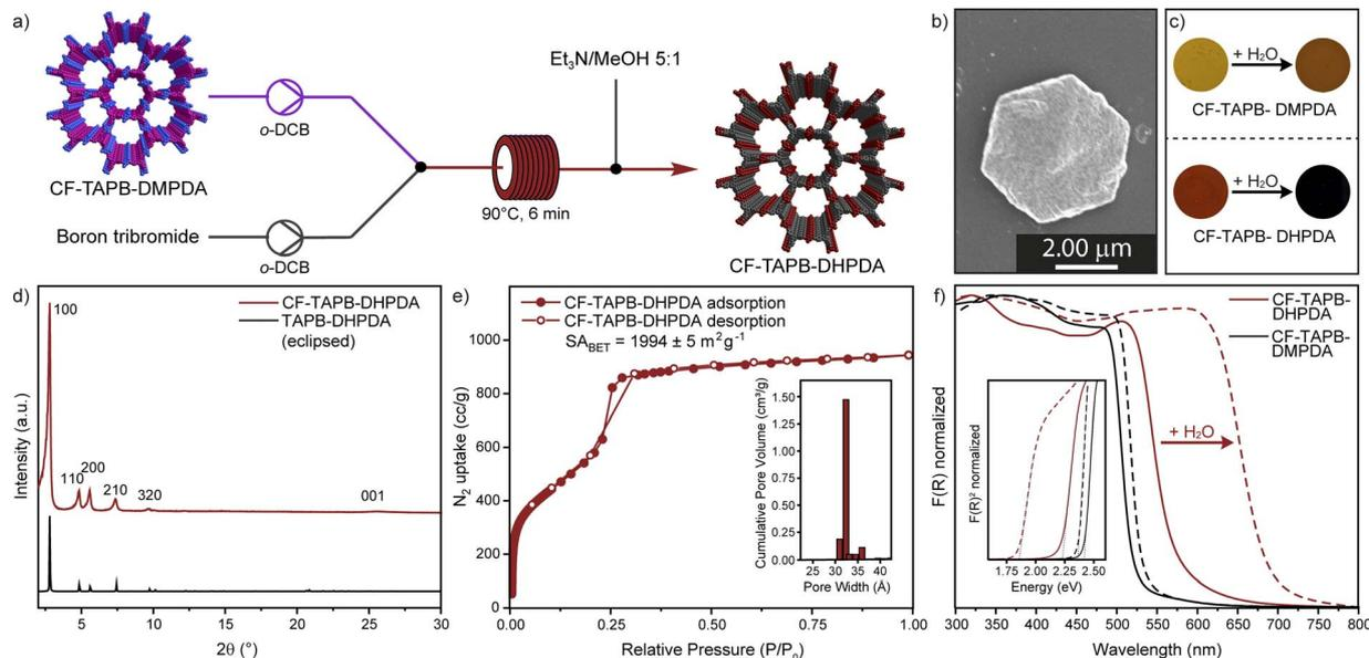
Fig. 4 Continuous flow post-synthetic single crystal to single crystal conversion of CF-TAPB-DMPDA (a). Scanning electron microscopy image (b). Optical image of methylated and demethylated COF before and after dispersion in water (c). PXRD (d) and nitrogen isotherms with pore size distribution in the inlet of CF-TAPB-DHPDA (e). UV-vis spectroscopy with Tauc plot in the inlet of methylated and demethylated COF before and after dispersion in water (f).
