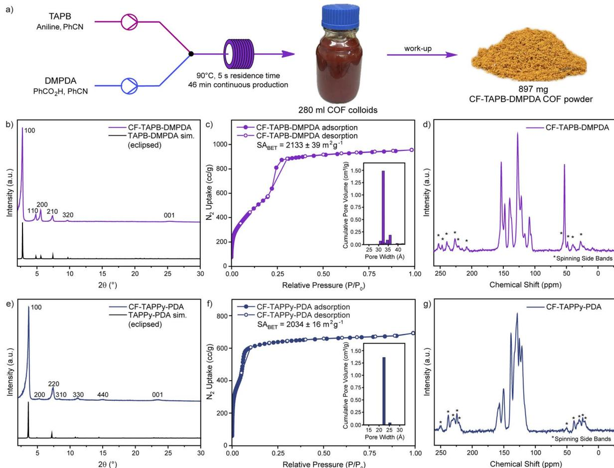
Fig. 3 Scaled-up continuous production of CF-TAPB-DMPDA (a). PXRD (b), nitrogen isotherms with pore size distribution in the inlet (c) and  $^{13}\text{C}$  solid state NMR analysis (d) of scaled-up CF-TAPB-DMPDA. PXRD (e), nitrogen isotherms with pore size distribution in the inlet (f) and  $^{13}\text{C}$  solid state NMR analysis (g) of scaled-up CF-TAPPy-PDA.
