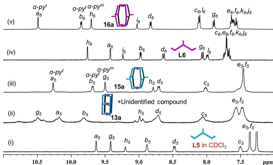
**Fig. 5** Partial  $^1\text{H}$  NMR spectra (400 MHz, DMSO- $d_6$ , 300 K) of (i) ligand L5 (in  $\text{CDCl}_3$ ); (ii)  $[\text{Pd}_3(\text{L5})_4](\text{NO}_3)_6$ , **13a**, and unidentified complexes; (iii)  $[\text{Pd}_2(\text{L5})_4](\text{NO}_3)_4$ , **15a**; (iv) ligand L6; and (v)  $[\text{Pd}_2(\text{L6})_4](\text{NO}_3)_4$ , **16a**. (Note: spectrum (ii) corresponds to complexation reaction of  $\text{Pd}(\text{II})$  with ligand L5 in 3 : 4 ratio.).
