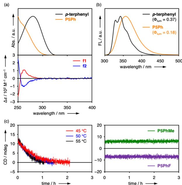
Fig. 4 (a) UV/vis absorption (top) and CD (bottom) spectra of P5Ph isomers (f1, f2) in  $\text{CHCl}_3$ . (b) FL spectra of P5Ph ( $\lambda_{\text{ex}} = 255 \text{ nm}$ ) and *p*-terphenyl ( $\lambda_{\text{ex}} = 280 \text{ nm}$ ) in  $\text{CHCl}_3$ . (c) Decay profiles of CD intensities at 260 nm for P5Ph at 45–55 °C in  $\text{CHCl}_3$  (left), and P5PhMe and P5PhF at 80 °C in 1,2-dichloroethane (right).
