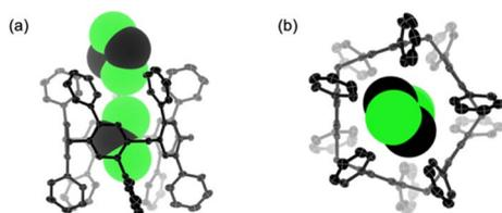
Fig. 2 X-ray crystal structure of **P5Ph**. (a) Side view and (b) top view. The molecule was obtained as a half structure in the asymmetric unit. Two dichloromethane molecules located at the special points were assigned without hydrogen atoms and are displayed with a space-filling model. Thermal ellipsoids are scaled to 50% probability and all hydrogen atoms are omitted for clarity. Element colours: black, carbon; light green, chlorine.
