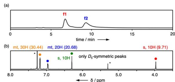
Fig. 3 (a) HPLC chart of *rac*-**P5Ph** recorded as absorption of 250 nm light. Conditions: CHIRALPAK IA ( $\phi = 4.6$  mm,  $l = 250$  mm) column; room temperature; flow rate = 1.0 mL min<sup>-1</sup>; eluent = CH<sub>2</sub>Cl<sub>2</sub>/*n*-hexane (1/10). (b) <sup>1</sup>H NMR (600 MHz) spectrum of an isolated fraction of **P5Ph** in CDCl<sub>3</sub> at 25 °C.
