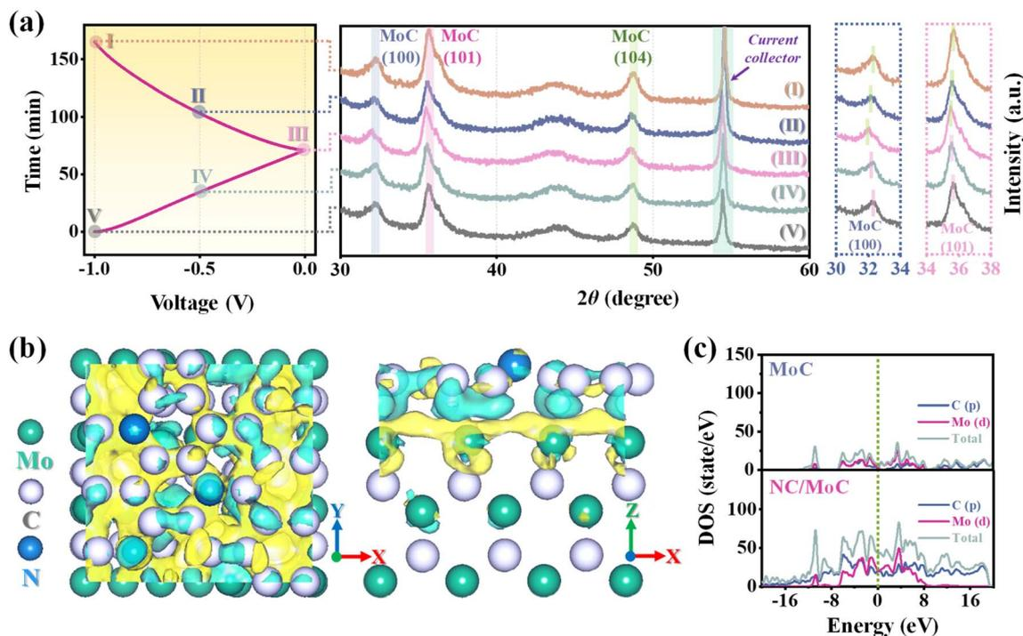
Fig. 5 (a) The charge/discharge curve and corresponding *ex situ* XRD patterns of NC/MoC-0.5 in various desalination/regeneration stages. (b) Differential charge density of the NC/MoC, where the reduction and increase in electron density are marked by green and yellow colors, respectively. (c) Electron density of states (DOS) of the NC/MoC and pure MoC.
