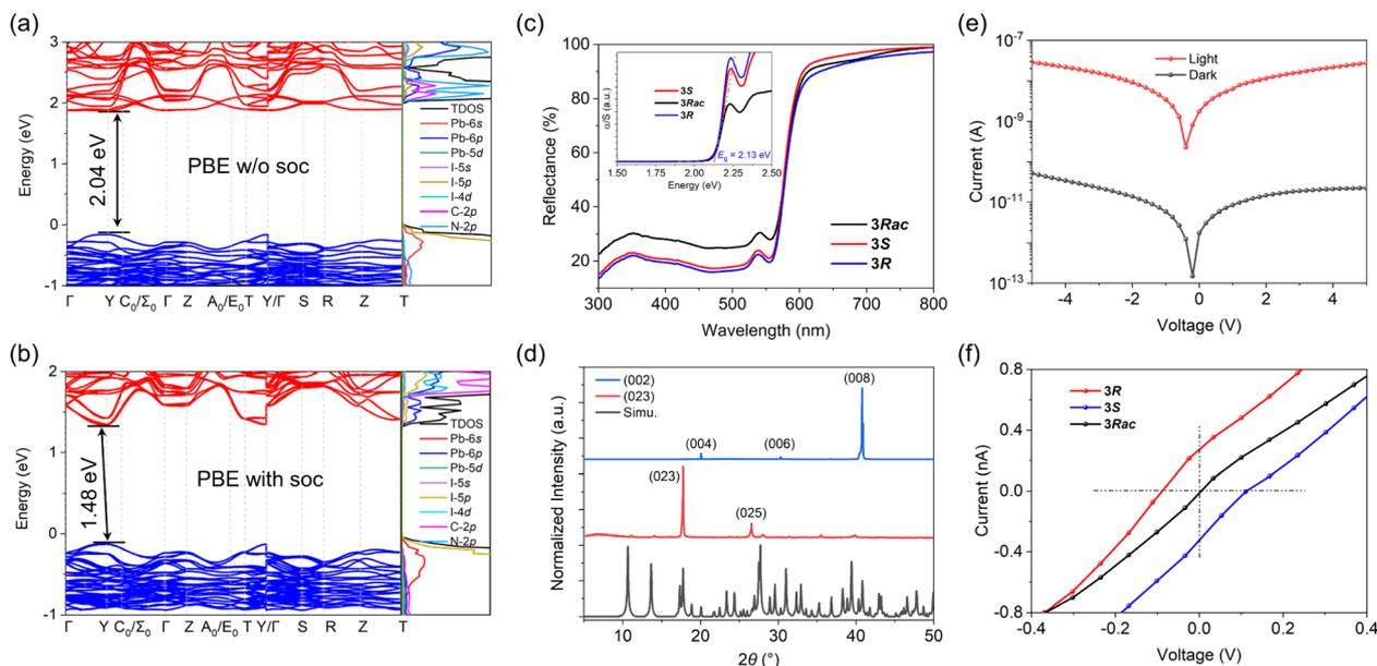
Fig. 3 (a) DFT-PBE and (b) DFT-PBE + SOC band structures and projected density of states (PDOS) of **3R**. (c) UV-vis diffuse-reflectance spectra of **3R/S/Rac**. Inset: optical bandgap derived from the Kubelka–Munk function based on diffuse-reflectance data. (d) PXRD patterns of the single crystal were recorded from the (023) and (001) planes. (e)  $I-V$  curves recorded in the dark and under  $100 \text{ mW cm}^{-2}$  illumination along the [100]. (f) Bulk photovoltaic effect of **3R/S**.
