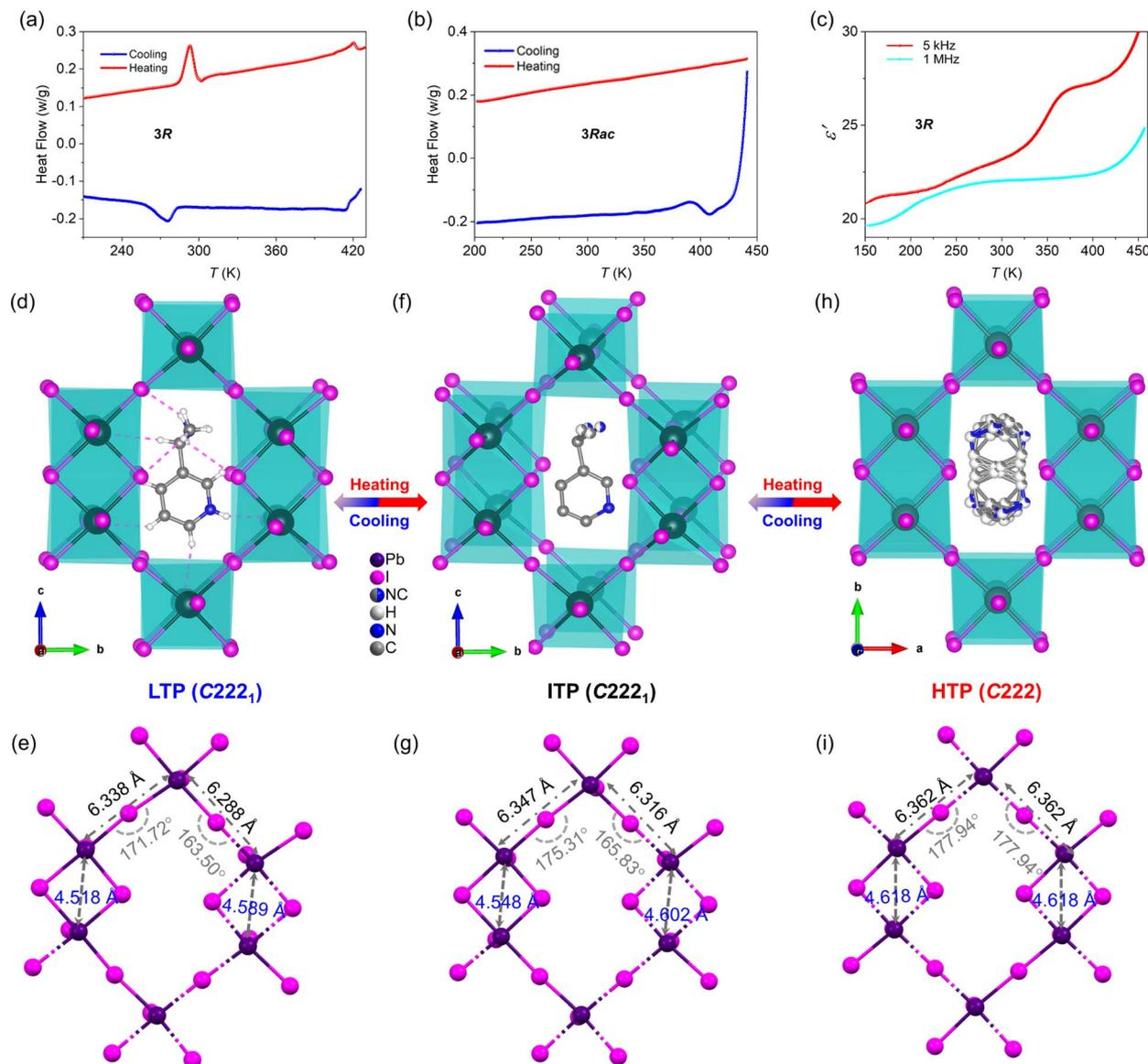
Fig. 2 (a) DSC curves of **3R**. (b) DSC curves of **3Rac**. (c) Dielectric transition of **3R**. Crystal structure of **3R** in the ordered LTP (d), and disordered ITP (f), HTP (h) and the corresponding connection motifs (e, g, and i).
