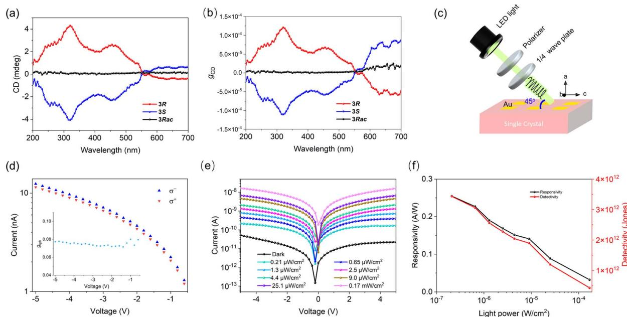
Fig. 4 (a) CD and (b)  $g_{CD}$  spectra of **3R/S** and **3Rac**. (c) Device architecture for the CPL detection of **3R**. (d)  $I-V$  curves of the **3R** photodetector under R-CPL and L-CPL illumination at 565 nm with an intensity of  $0.17 \text{ mW cm}^{-2}$ , as well as the calculated  $g_{lph}$ . (e)  $I-V$  curves under different illumination intensities at 565 nm; (f) power intensity dependence of  $R$  and  $D^*$  at 565 nm.
