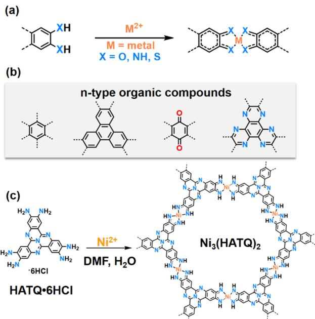
Fig. 1 The coordination of transition-metal ions with different planar conjugated ligands and design strategy of  $Ni_3(HATQ)_2$ . (a) The representative coordination process of square-planar transition-metal ions with *ortho*-substituted organic conjugated ligands. (b) The typical n-type organic structures in 2D *c*-MOFs. (c) The synthetic route of  $Ni_3(HATQ)_2$ .
