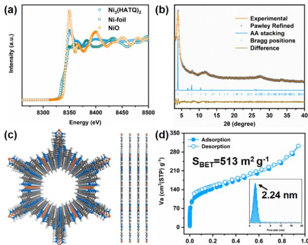
Fig. 2 Characterization of the valence state, crystallinity, simulated structure and porosity of Ni<sub>3</sub>(HATQ)<sub>2</sub>. (a) XANES of NiO, Ni foil and Ni<sub>3</sub>(HATQ)<sub>2</sub>. (b) Experimental and Pawley refined XRD profiles of Ni<sub>3</sub>(HATQ)<sub>2</sub>. (c) The structural model. (d) Nitrogen-sorption isotherms of Ni<sub>3</sub>(HATQ)<sub>2</sub>.
