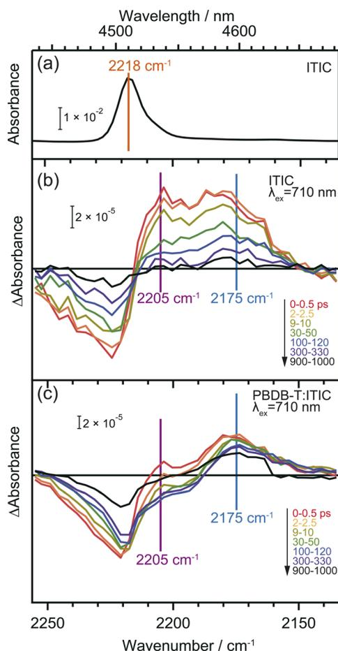
Fig. 4 Vibrational spectra of CN groups in ITIC. Steady-state FT-IR spectrum of neat ITIC film (a). Transient IR absorption spectra of neat ITIC film (b) and PBDB-T:ITIC blend film (c) irradiated by  $710\text{ nm}$  pump pulse. Broad absorption by photocarriers was subtracted to extract the change of CN vibrations.
