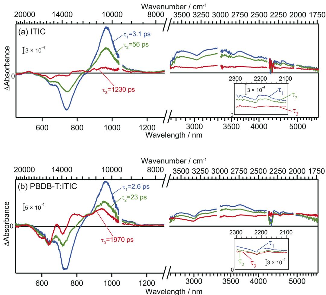
Fig. 3 Global analysis of the transient absorption spectra of neat ITIC (a) and PBDB-T:ITIC blend film (b). Inset is the enlarged view around 2200 cm<sup>-1</sup>.
