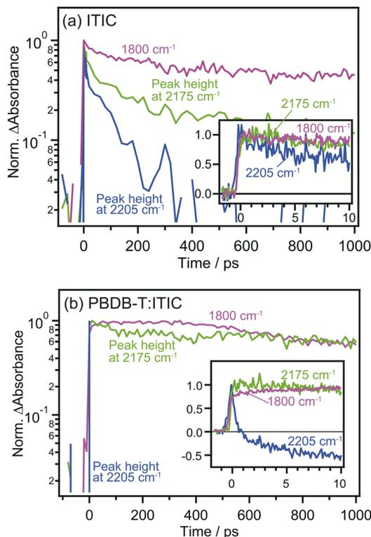
Fig. 5 Time profiles of excited  $S_1$  state, anionic ITIC, and free electrons measured at 2205, 2175, and 1800  $\text{cm}^{-1}$  in neat ITIC (a) and PBDB-T:ITIC blend films (b), respectively. The peak heights at 2205 and 2175  $\text{cm}^{-1}$  were calculated after subtracting the broad absorptions by photocarriers to extract the change of CN vibrations.
