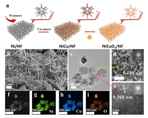
Fig. 1 (a) Synthesis of NiCuO<sub>x</sub>/NF (schematic). (b) SEM, (c) TEM, (d and e) HRTEM images and (f-i) EDS elemental mappings of NiCuO<sub>x</sub>-2/NF.
