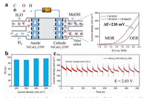
Fig. 5 (a) Scheme for a two-electrode electrolyzer for concurrent electrolytic production of hydrogen and value-added chemicals, and LSV curves of NiCuO<sub>x</sub>-2/NF in KOH (1.0 M) with and without addition of methanol (1 M). (b) FEs of generated formate at the anode after operating at 200, 300, 400 and 500 mA cm<sup>-2</sup> for 1 h. (c) Chronoamperometry (l-t) curves by NiCuO<sub>x</sub>-2/NF-equipped MOR||HER at a constant potential of 2.03 V.
