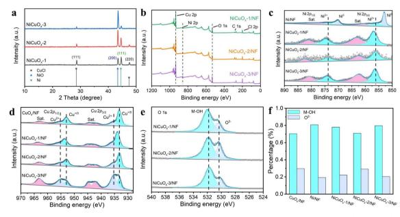
Fig. 2 (a) XRD patterns for NiCuO<sub>x</sub>-1, NiCuO<sub>x</sub>-2 and NiCuO<sub>x</sub>-3. Survey XPS spectrum (b), high-resolution XPS Ni 2p (c), Cu 2p (d), O 1s (e) and corresponding histograms (f) of M-OH/O<sup>2-</sup> sub-bands for as-prepared catalysts.
