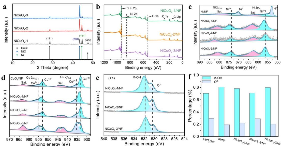
Fig. 2 (a) XRD patterns for NiCuO<sub>x</sub>-1, NiCuO<sub>x</sub>-2 and NiCuO<sub>x</sub>-3. Survey XPS spectrum (b), high-resolution XPS Ni 2p (c), Cu 2p (d), O 1s (e) and corresponding histograms (f) of M-OH/O<sup>2-</sup> sub-bands for as-prepared catalysts.
