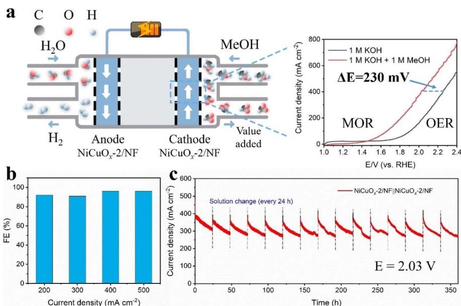
Fig. 5 (a) Scheme for a two-electrode electrolyzer for concurrent electrolytic production of hydrogen and value-added chemicals, and LSV curves of NiCuO<sub>x</sub>-2/NF in KOH (1.0 M) with and without addition of methanol (1 M). (b) FEs of generated formate at the anode after operating at 200, 300, 400 and 500 mA cm<sup>-2</sup> for 1 h. (c) Chronoamperometry (*I*–*t*) curves by NiCuO<sub>x</sub>-2/NF-equipped MOR||HER at a constant potential of 2.03 V.
