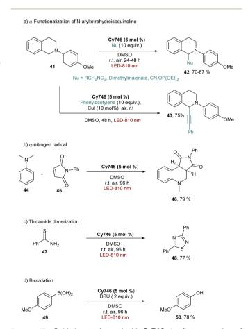
Scheme 13 Oxidation performed with Cy746, the first generation of cyanine-based NIR-photocatalysts.
