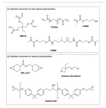
Scheme 11 Selected examples of monomers compatible with cyanine-based NIR photopolymerization.
