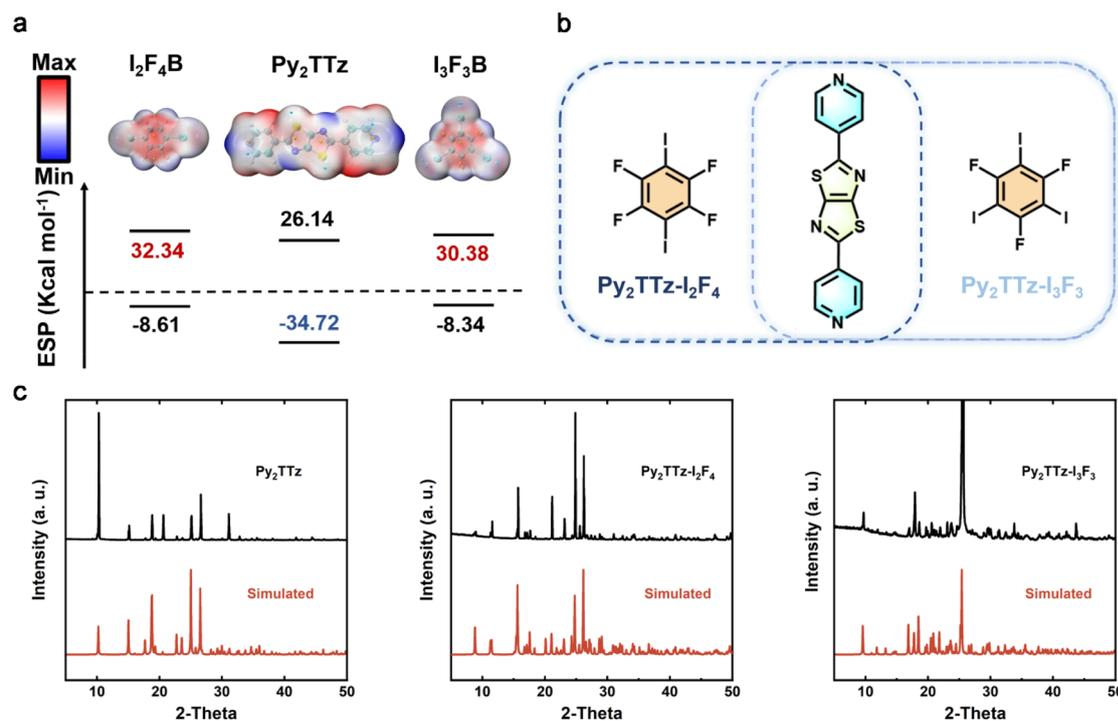
Fig. 1 (a) Calculated molecular electrostatic surface potential (ESP) visualization and extreme values for Py<sub>2</sub>TTz, I<sub>2</sub>F<sub>4</sub>B, and I<sub>3</sub>F<sub>3</sub>B. (b) Chemical structures of Py<sub>2</sub>TTz-I<sub>2</sub>F<sub>4</sub> and Py<sub>2</sub>TTz-I<sub>3</sub>F<sub>3</sub>. (c) XRD patterns of Py<sub>2</sub>TTz, Py<sub>2</sub>TTz-I<sub>2</sub>F<sub>4</sub> and Py<sub>2</sub>TTz-I<sub>3</sub>F<sub>3</sub> crystalline powders compared with simulated XRD patterns.
