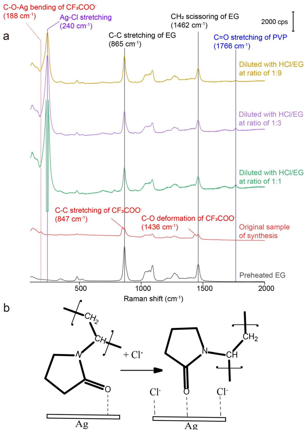
Fig. 5 (a) Raman spectrum of preheated EG and SERS spectra recorded from the original reaction solution of Ag irregular particles synthesized using  $\text{CF}_3\text{COOAg}$  and after it had been diluted with  $\text{HCl/EG}$  at various ratios, with the final concentration of  $\text{Cl}^-$  being  $0.21\text{ mM}$ ; and (b) schematic showing the effect of chemisorbed  $\text{Cl}^-$  on the orientation of  $\text{C=O}$  group of PVP relative to the Ag surface.
