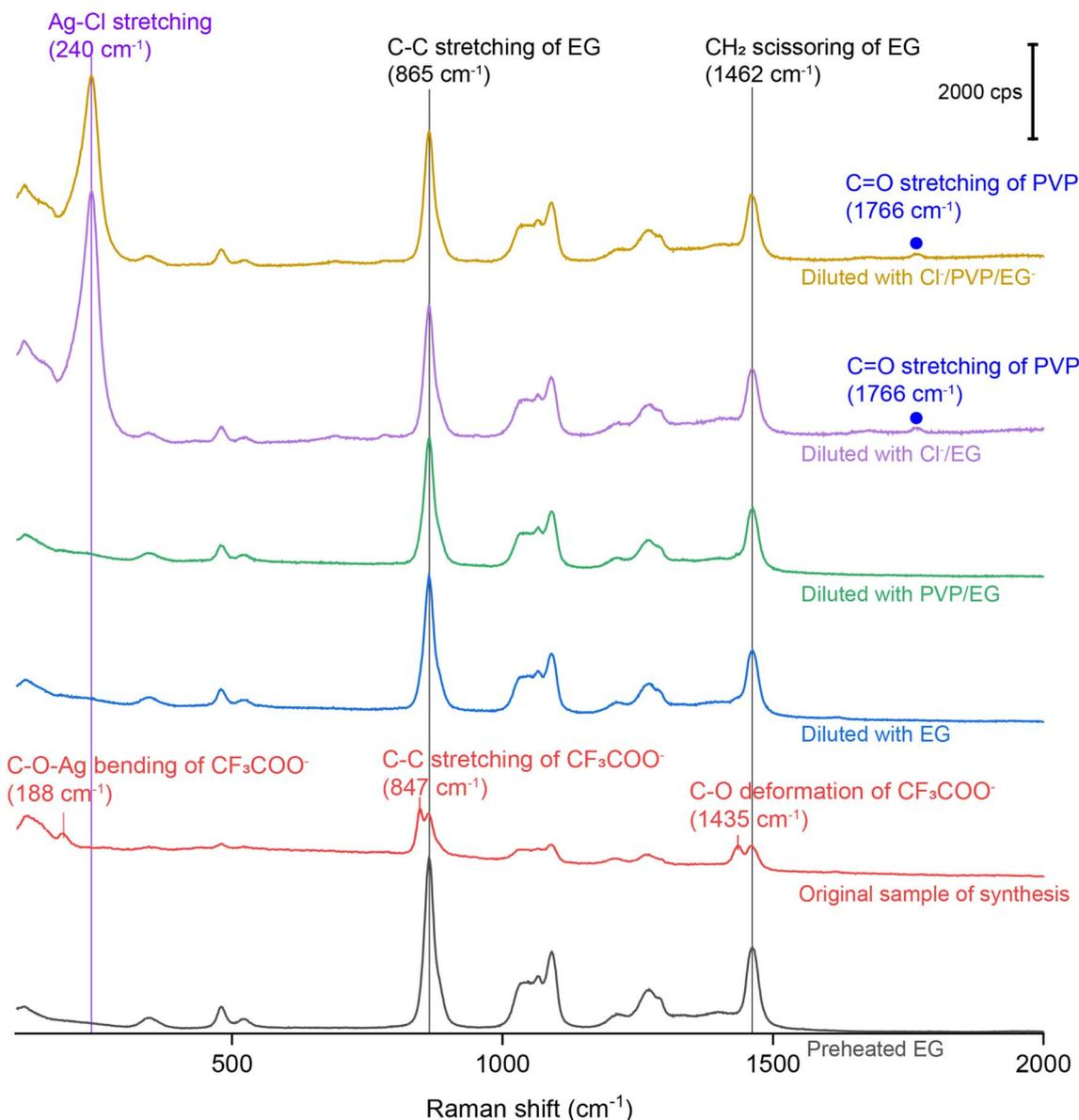
Fig. 3 Raman spectrum of the preheated EG, SERS spectra of the as-obtained Ag irregular particles in the original reaction solution containing no Cl<sup>-</sup> and after it had been diluted by 10 times with EG, EG containing PVP, EG containing Cl<sup>-</sup>, and EG containing both PVP and Cl<sup>-</sup>.
