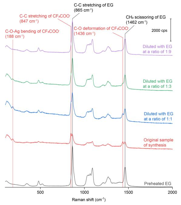
Fig. 4 Raman spectrum of preheated EG and SERS spectra recorded from the original reaction solution of Ag irregular particles synthesized using CF<sub>3</sub>COOAg and after it had been diluted with the EG at various ratios.
