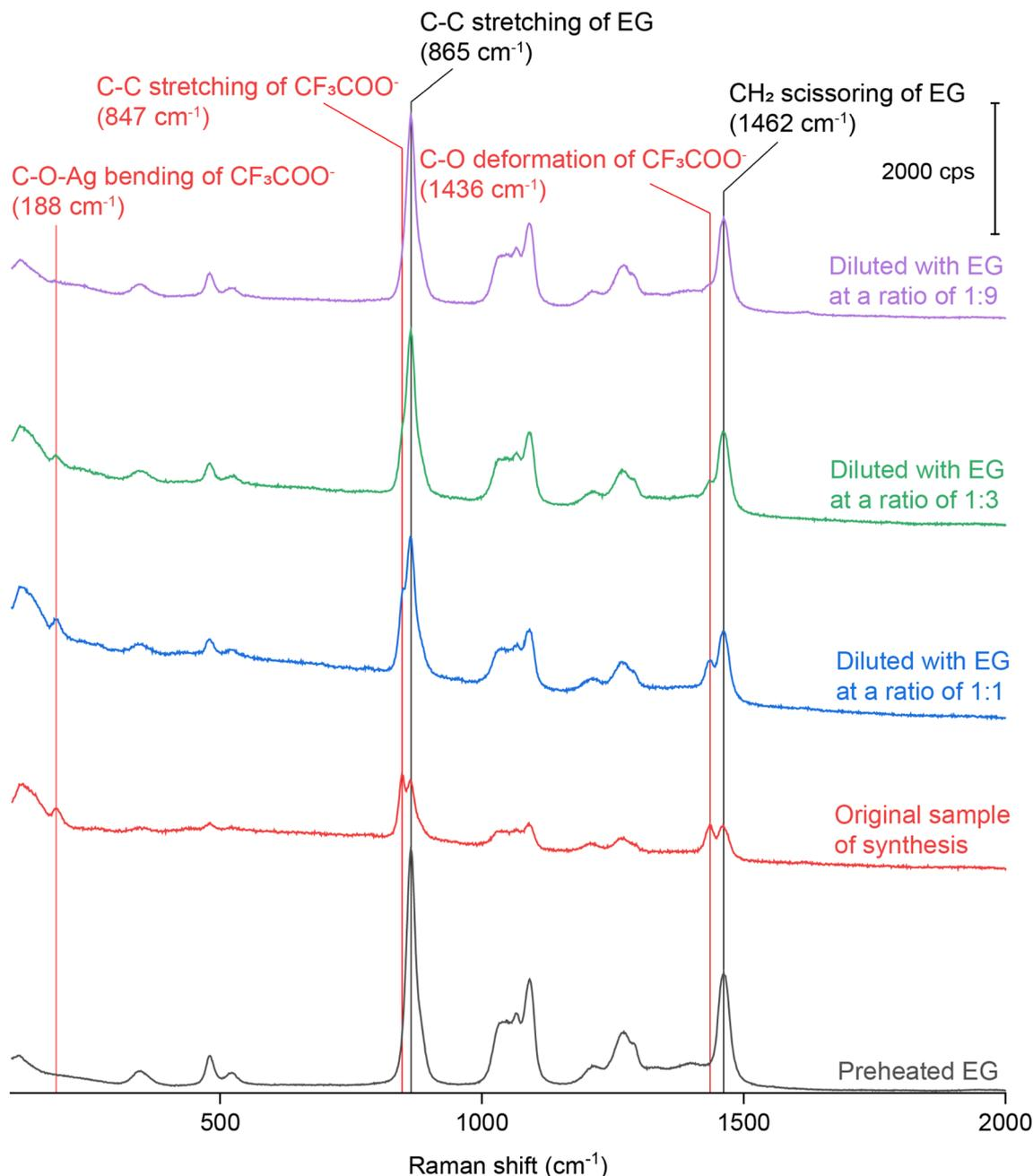
Fig. 4 Raman spectrum of preheated EG and SERS spectra recorded from the original reaction solution of Ag irregular particles synthesized using CF<sub>3</sub>COOAg and after it had been diluted with the EG at various ratios.
