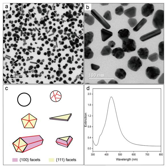
Fig. 2 (a and b) TEM images of the Ag irregular particles prepared in the absence of Cl<sup>-</sup>, which were collected by precipitation with acetone, followed by centrifugation and washing with water. (c) Models showing the typical shapes (with the facets color coded) taken by the nanocrystals. The twin boundaries are marked by red lines. (d) UV-vis spectrum recorded from a suspension of the Ag nanocrystals in the original reaction solution.
