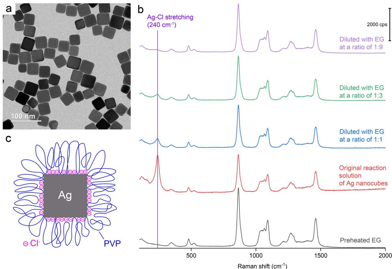
**Fig. 1** (a) A typical TEM image of the Ag nanocubes. (b) Raman spectrum of EG (preheated at 150 °C for 1 h) and SERS spectra recorded from the original reaction solution of Ag nanocubes and after it had been diluted with preheated EG at various ratios. (c) A model detailing the native surface of a Ag nanocube suspended in the original reaction solution.
