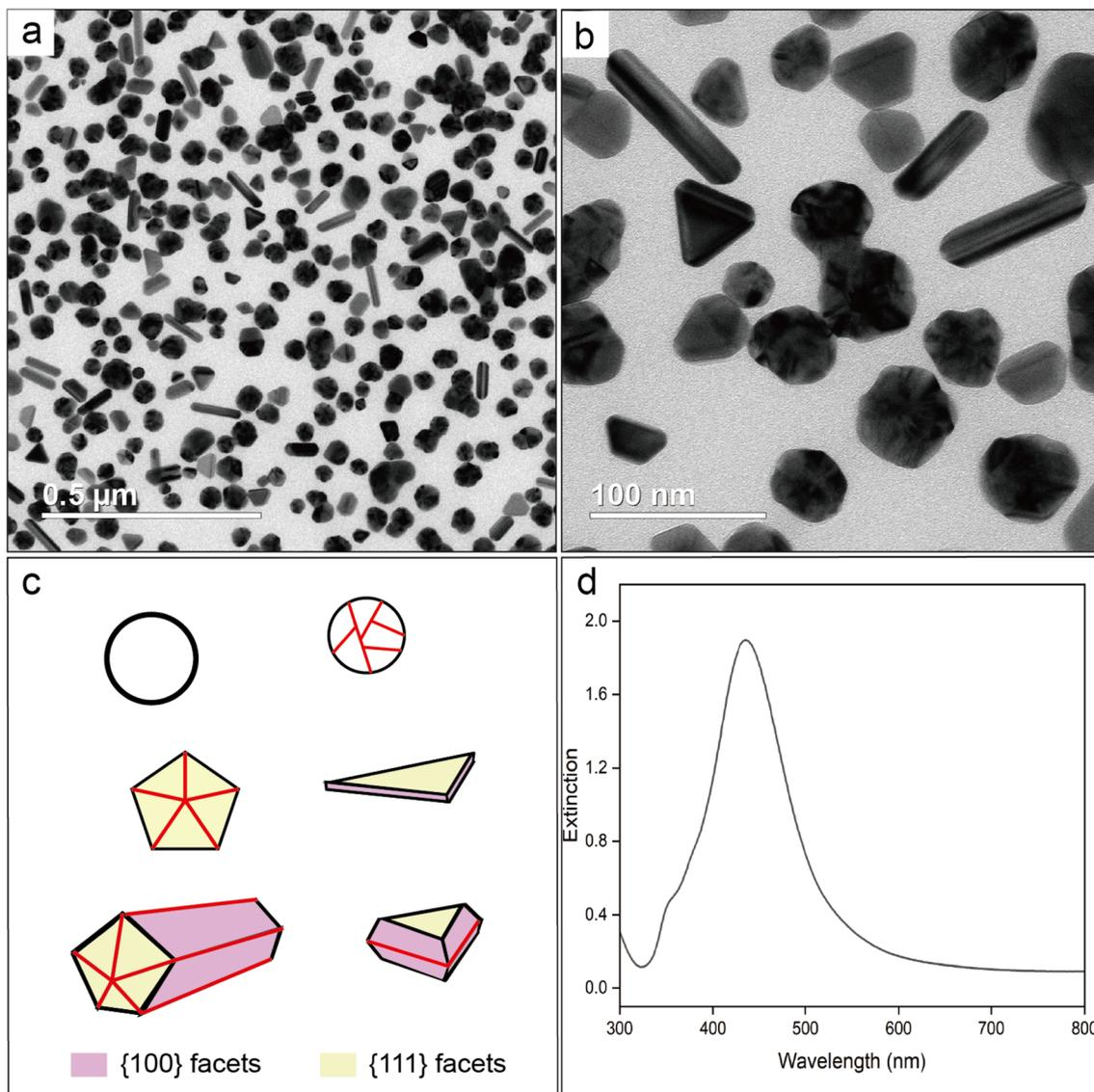
Fig. 2 (a and b) TEM images of the Ag irregular particles prepared in the absence of  $\text{Cl}^-$ , which were collected by precipitation with acetone, followed by centrifugation and washing with water. (c) Models showing the typical shapes (with the facets color coded) taken by the nanocrystals. The twin boundaries are marked by red lines. (d) UV-vis spectrum recorded from a suspension of the Ag nanocrystals in the original reaction solution.
