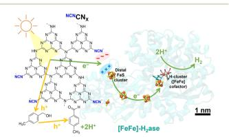
Fig. 1 Schematic of photocatalytic H<sub>2</sub> evolution coupled with alcohol oxidation to aldehyde using an electrostatic  $^{NCN}CN_X|[FeFe]-H_2$ ase (CpI, PDB: 4XDC) assembly. Scale bar refers to enzyme and  $CN_X$  is not shown to scale
