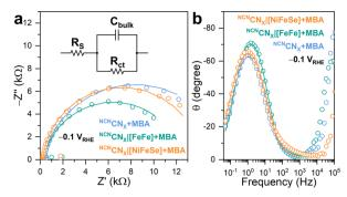
Fig. 4 (a) Nyquist plots and (b) Bode phase plots of PEIS signal (open circles) with corresponding fitting curves (solid lines). Inset: proposed equivalent circuit to fit the impedance response. Conditions: 20 mL anaerobic MOPS buffer (0.1 M, pH 7) containing 50 mM 4-MBA, Ag/AgCl (3 M NaCl) reference electrode, Pt mesh counter electrode, AM 1.5G irradiation, 25 °C.
