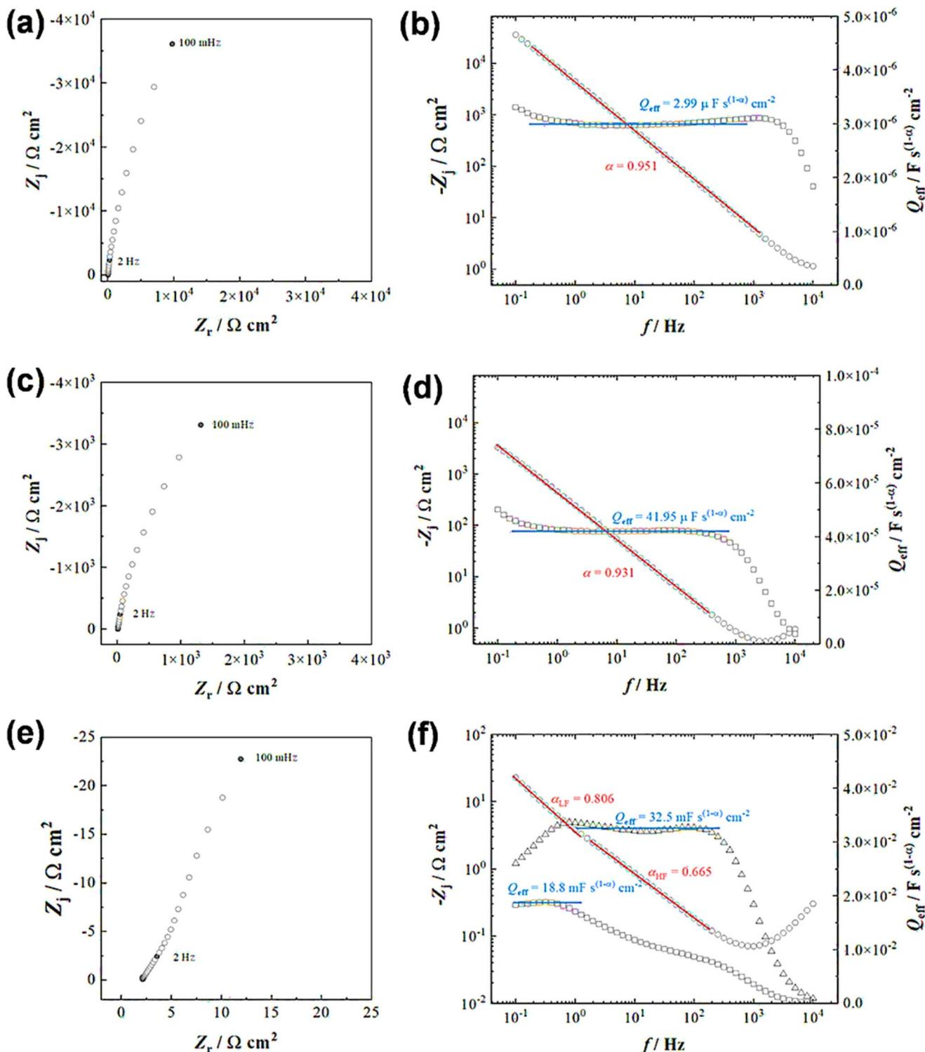
Fig. 5 Electrochemical impedance responses and graphical analysis for the determination of CPE parameters on (a and b) the bare electrode, (c and d) ANT-modified GR, and (e and f) after  $10^4$  GCD cycles at +0.3 V (vs. Ag/AgCl in 1 M  $\text{H}_2\text{SO}_4$ ).
