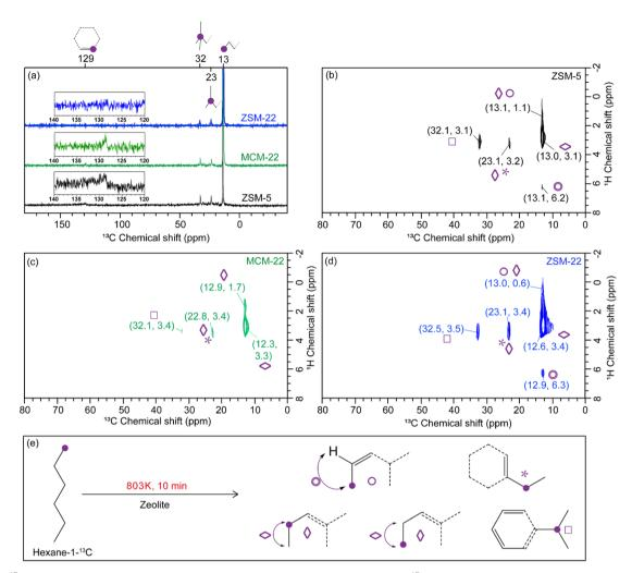
Fig. 4 The  $^{13}$ C NMR solid-state spectra of zeolite-trapped organics after the hexane- $1^{-13}$ C conversion over zeolites ZSM-5 (black), MCM-22 (green) and ZSM-22 (blue) (MAS = 16 kHz): (a) 1D  $^{1}$ H- $^{13}$ C cross-polarization (CP) MAS spectra of all three zeolites and (b-d) 2D  $^{1}$ H- $^{13}$ C CP HETCOR MAS spectra of post-reacted zeolites (b) ZSM-5, (c) MCM-22, and (d) ZSM-22. (e) Identified molecular scaffolds (also see Fig. S17†).
