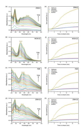
Fig. 3 Operando mechanistic study: (a–d) time-monitored UV-vis DRS profile and (e–h) time-resolved mass-spectral profiles of key hydrocarbon effluent species during the catalytic *n*-hexane conversion over zeolites ZSM-5 (a and e), MCM-22 (b and f), FER (c and g) and ZSM-22 (d and h) for 20 min at 803 K.
