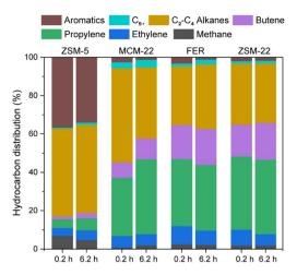
Fig. 2 Hydrocarbon distribution in the effluent gas phase over ZSM-5, MCM-22, FER, and ZSM-22 zeolites during early (first GC injection:  $\sim$ 0.2 h for *n*-hexane catalytic cracking conversion) and steady states (~6.2 h) of reaction (reaction conditions: 803 K, 1 atm). Also, see Fig. S9-S12† for additional catalysis data.
