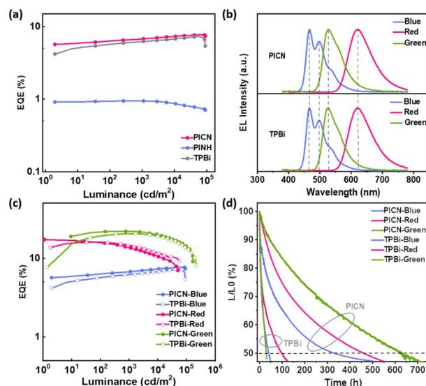
Fig. 3 Performances of OLEDs with different ETMs. (a) EQE– $L$  curves of the blue FOLEDs based on three different ETMs. (b) EL spectra at 4 V of the devices with **PICN** and **TPBi** as the ETMs. (c) EQE– $L$  curves of the devices with **PICN** and **TPBi** as the ETMs. (d) Lifetime curves of the devices with **PICN** and **TPBi** as the ETMs at a fixed current density with an  $L_0$  of  $1000 \text{ cd m}^{-2}$ .
