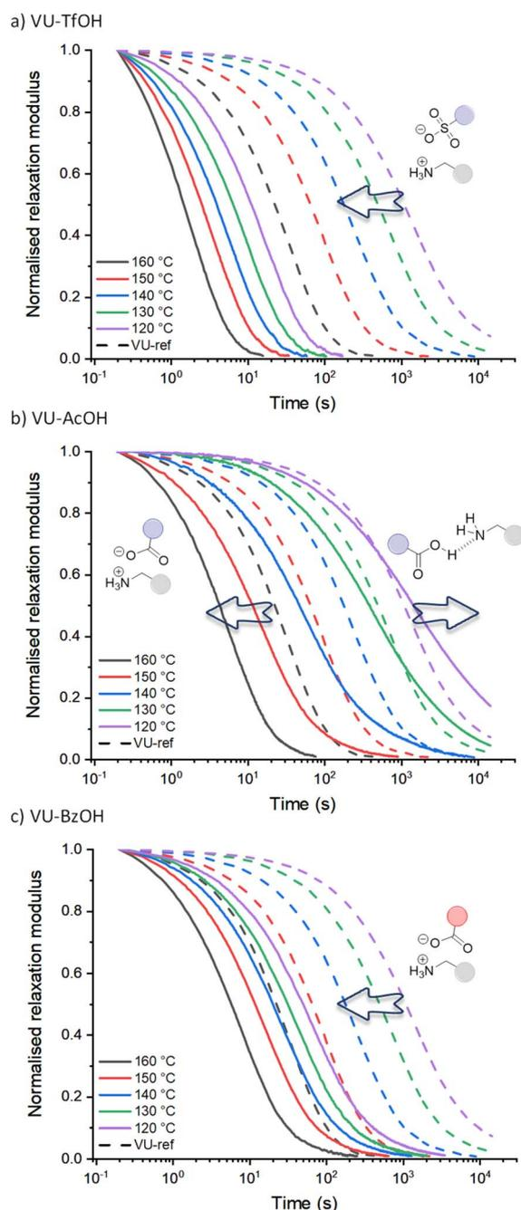
Fig. 3 Normalised stress-relaxation curves of (a) VU-TfOH, (b) VU-AcOH and (c) VU-BzOH measured from  $160$  to  $120$  °C and compared to VU-ref (dashed lines). Different viscoelastic behaviour could be observed depending on the acid strength of the additive.
