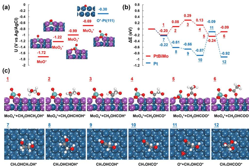
Fig. 6 (a) Calculated onset potentials for the oxidation of surface Mo atoms by adsorbed O to form MoO, MoO<sub>2</sub>, MoO<sub>3</sub>, and MoO<sub>4</sub>, respectively, with optimized structures. (b) Energy profiles for the ethylene glycol electrooxidation to glycolate on PtBiMo (red lines) and Pt (blue lines). (c) Optimized intermediate structures on PtBiMo and Pt. blue: Pt; purple: Bi; green: Mo; grey: C; white: H; red: O.
