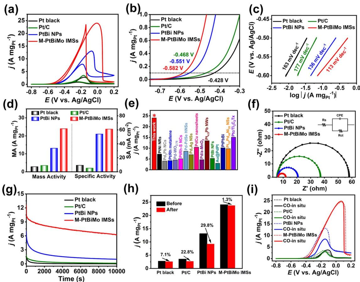
Fig. 3 (a and b) CV curves. (c) Tafel plots. (d) MA and SA. (e) Comparison of MA reported for various Pt/Pd-based EGOR catalysts. (f) Nyquist plots. (g)  $I-t$  curves recorded at  $-0.25$  V. (h) Normalized MA of commercial Pt black, Pt/C, PtBi NPs, and M-PtBiMo IMSs before and after the  $I-t$  test. (i) CV curves of Pt black, Pt/C, PtBi NPs, and M-PtBiMo IMSs in CO-saturated electrolyte.
