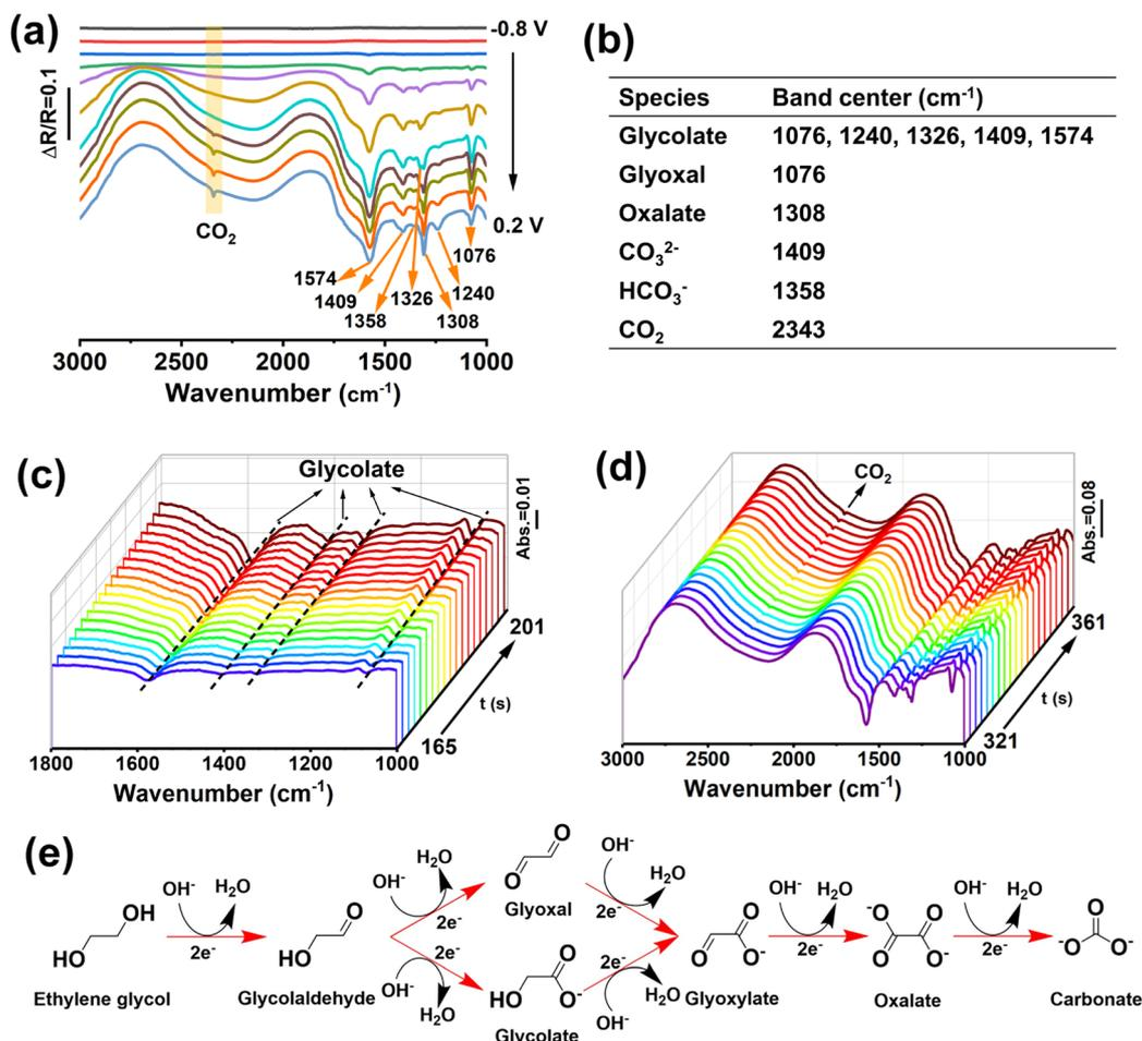
Fig. 4 (a) *In situ* FTIR spectra of M-PtBiMo IMSs in 1 M KOH + 1 M EG. (b) IR bands and their assignment for the EGOR. Real-time *in situ* FTIR spectra of M-PtBiMo IMSs at (c)  $-0.5$  V and (d)  $-0.1$  V, with an interval of 2 s. (e) Schematic of the proposed reaction pathways for the EGOR at the M-PtBiMo IMSs in alkaline media.
