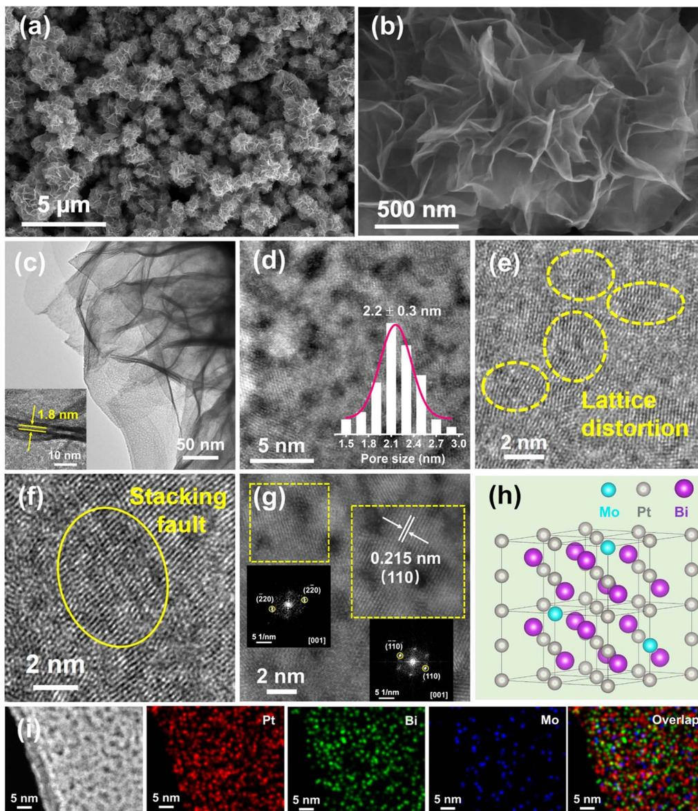
**Fig. 1** (a and b) SEM images of M-PtBiMo IMSs. (c) TEM image of M-PtBiMo IMSs. (d) High-resolution HAADF-STEM image (the inset shows the column chart of the size of pores) of M-PtBiMo IMSs. (e and f) High-resolution TEM images of M-PtBiMo IMSs. (g) High-resolution HAADF-STEM image (the inset shows the corresponding FFT patterns) of M-PtBiMo IMSs. (h) Crystal structure. (i) HAADF-STEM pattern and element mappings of M-PtBiMo IMSs.
