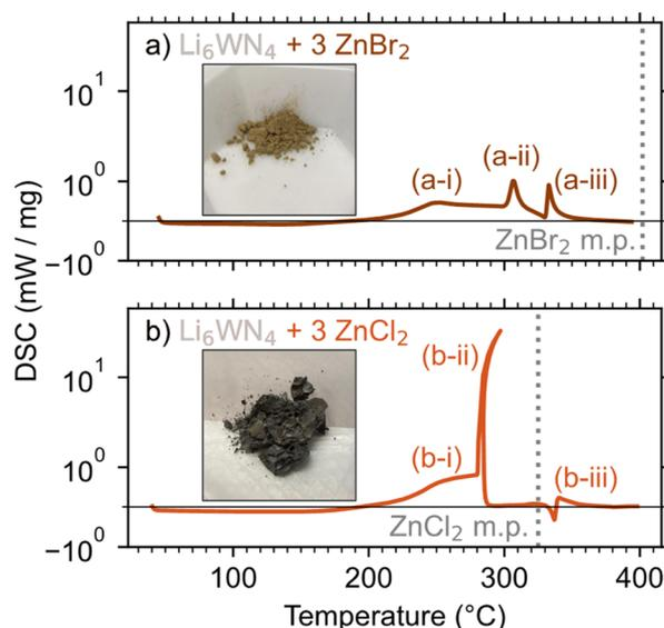
Fig. 3 DSC measurements of  $\text{Li}_6\text{WN}_4$  reacting with (a) 3  $\text{ZnBr}_2$  and (b) 3  $\text{ZnCl}_2$ . Inset photos show the products from reactions with  $\text{Zn}$  heated at 300 °C for 1 h.
