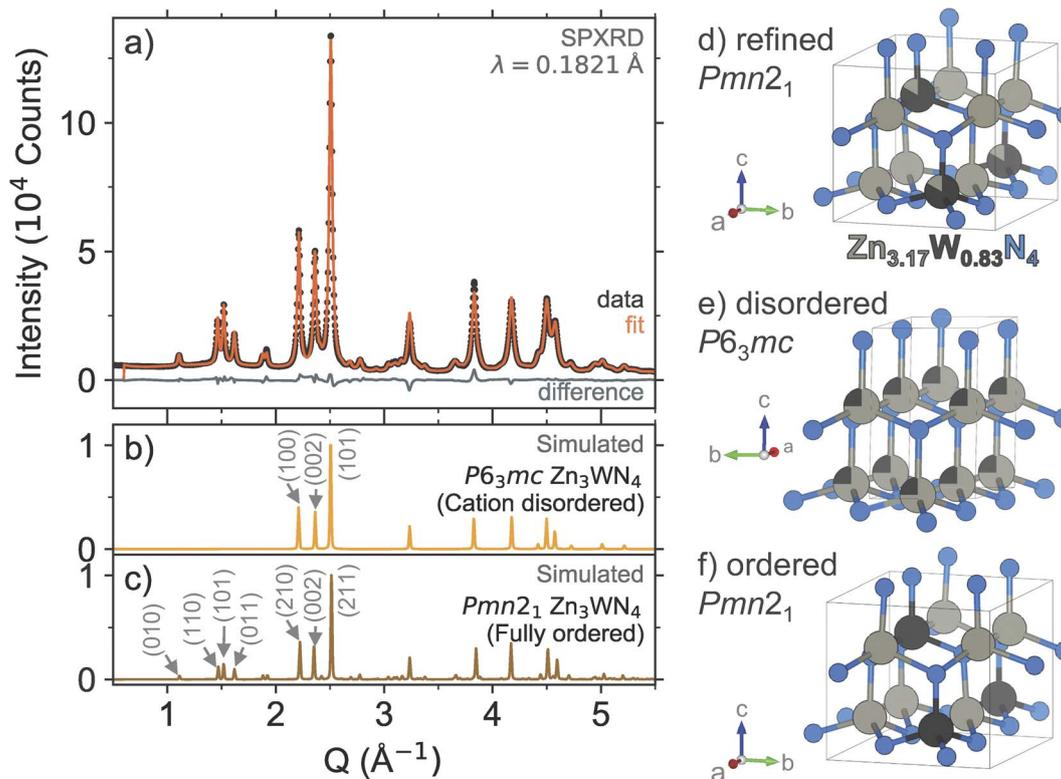
Fig. 5 (a) High resolution SPXRD data (black dots) and Rietveld refinement (orange trace) of  $\text{Zn}_{3.17}\text{W}_{0.83}\text{N}_4$  powder. Simulated patterns are shown for reference: (b) the cation-disordered  $P6_3mc$  model and (c) the fully ordered  $Pmn2_1$  model. Visualizations of (d) the  $Pmn2_1$  structure of  $\text{Zn}_{3.17}\text{W}_{0.83}\text{N}_4$  refined from the SPXRD data, (e) the cation-disordered  $P6_3mc$  model, and (f) the fully ordered  $Pmn2_1$  model.
