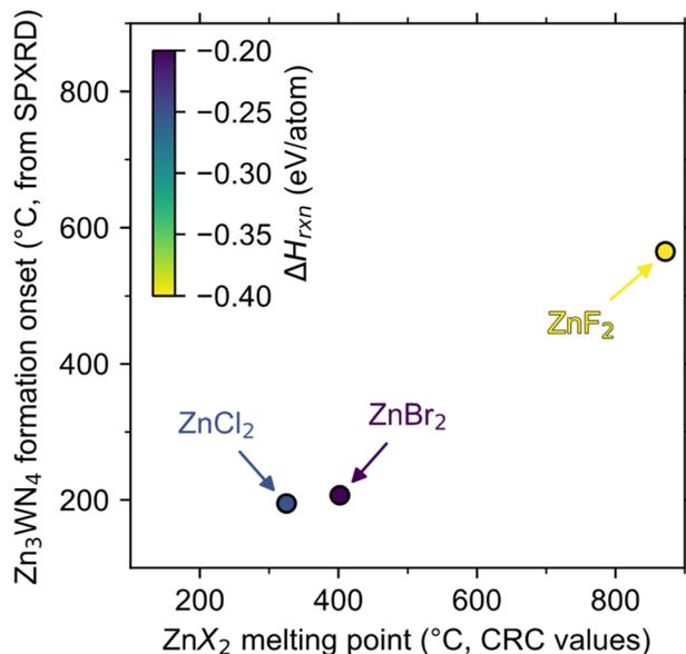
Fig. 4 The initial formation of  $\text{Zn}_3\text{WN}_4$  (as detected by *in situ* SPXRD) is correlated with the melting point of the halide salt (from CRC values)<sup>50</sup> but is not correlated with calculated reaction enthalpy ( $\Delta H_{\text{rxn}}$ , color, from the materials project).<sup>84</sup> The dashed line shows where melting point would equal onset temperature.
