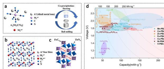
Fig. 4 Cathodes based on Prussian blue analogues. (a) The schematic diagram of PBA preparation; (b) the ideal structures of cubic PBAs; (c) the ideal rhombohedral structures of  $\text{ZnHCF}$ . Adapted from ref. 74, copyright 2022, Elsevier Ltd. (d) Comparison of PBAs applied to AZIBs. Adapted from ref. 75, copyright 2024, The Royal Society of Chemistry.
