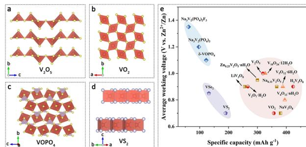
Fig. 2 Vanadium-based cathodes. The crystal structures of (a) V<sub>2</sub>O<sub>5</sub>, (b) VO<sub>2</sub>, (c) VOPO<sub>4</sub> and (d) VS<sub>2</sub>. (e) Average working voltages versus specific capacities of representative vanadium-based cathode materials for AZIBs. Data from ref. 29, 32, 35 and 37–49.
