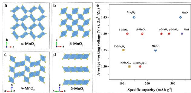
Fig. 3 Manganese-based cathodes. The crystal structures of (a)  $\alpha$ - $\text{MnO}_2$ , (b)  $\beta$ - $\text{MnO}_2$ , (c)  $\gamma$ - $\text{MnO}_2$ , (d)  $\delta$ - $\text{MnO}_2$ . (e) Average working voltages versus specific capacities of representative manganese-based cathode materials for AZIBs. Data from ref. 54, 55, 57, 58, 60, 61 and 63–67.
