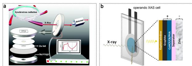
Fig. 12 X-ray *in situ* cells for the study of cathode materials in AZIBs. (a) Schematic diagram of the *operando* synchrotron radiation X-ray test cells and measurement environment. Adapted from ref. 155, copyright 2021, The Royal Society of Chemistry. (b) Schematic diagram of the XAS cell setup, consisting of a pouch cell with an X-ray transparent Kapton window. Adapted from ref. 156, copyright 2021, The Authors. Published by American Chemical Society.
