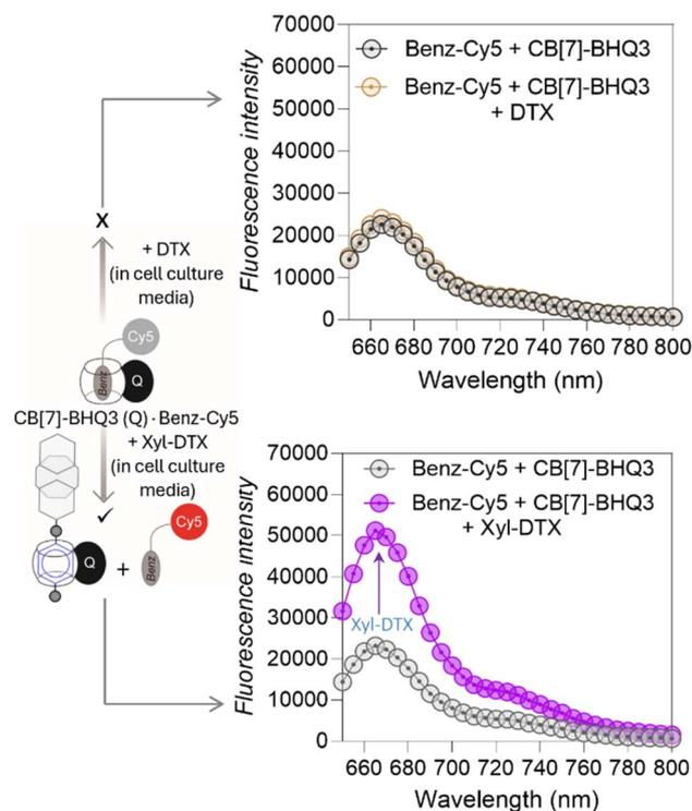
Fig. 3 Displacement assay to study complexation of CB[7] and Xyl-DTX in cell culture media. The addition of Xyl-DTX (10  $\mu\text{M}$ ) to a quenched solution of CB[7]-BHQ3 · Benz-Cy5 complex (prepared by mixing 1  $\mu\text{M}$  of CB[7]-BHQ3 and 1  $\mu\text{M}$  of Benz-Cy5) resulted in fluorescence recovery, indicating that Xyl-DTX displaced Benz-Cy5 and formed a CB[7]-BHQ3 · Xyl-DTX complex. No fluorescence recovery was observed upon the addition of DTX (10  $\mu\text{M}$ ).
