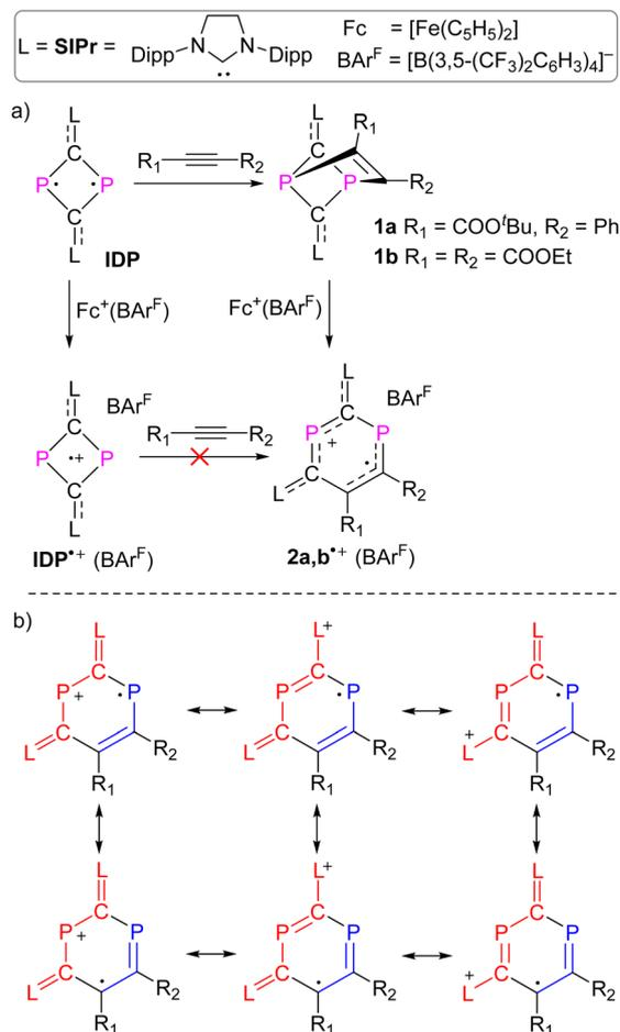
Scheme 1 (a) Synthesis of compounds **1** and **2**<sup>+</sup>(BAR<sup>F</sup>); (b) selected resonance structures of DRC **2**<sup>+</sup> in order to indicate delocalization of the positive charge in the red part of the molecule and delocalization of the spin in the blue area.
