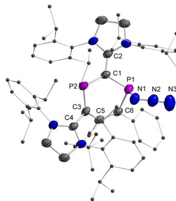
**Fig. 8** Plots of the molecular structure of  $6^+(\text{BAR}^{\text{F}})$  (ellipsoids are set to 50% probability; H atoms, anions, and solvents are omitted for clarity). Selected distances ( $\text{\AA}$ ):  $6^+$ : P1–N1 1.775(3), N1–N2 1.215(5), N2–N3 1.142(6), P1–C1 1.794(3), P1–C6 1.814(4), C6–C5 1.359(5), C5–C3 1.483(4), C3–P2 1.723(4), P2–C1 1.746(4), C1–C2 1.415(5), and C3–C4 1.470(5).
