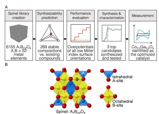
Fig. 1 (A) Scheme describing the computational workflow to identify new catalysts for OER. In this workflow,  $Co_{2.5}Ga_{0.5}O_4$  was discovered as a highly-performing spinel oxide catalyst. (B) Diagram describing the structure of a spinel oxide  $AB_2O_4$ , where A is tetrahedrally coordinated and B is octahedrally coordinated.
