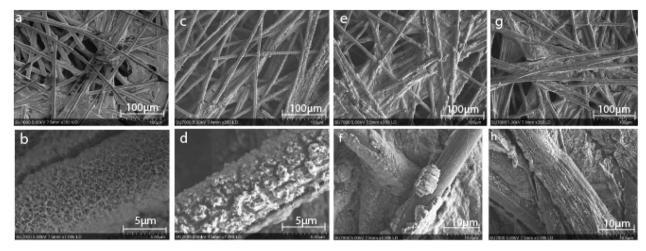
Fig. 4 SEM images of all four catalysts with two different resolutions. The four images on the top show zoomed out images of catalysts presumed to be (a)  $Co_3O_4$ , (c)  $Co_{1.5}Al_{1.5}O_4$ , (e)  $Co_{2.5}Ga_{0.5}O_4$  and (g)  $Co_{1.5}Ga_{1.5}O_4$ . The images at the bottom show zoomed in images of the same catalysts thought to be (b)  $Co_3O_4$ , (d)  $Co_{1.5}Al_{1.5}O_4$ , (f)  $Co_{2.5}Ga_{0.5}O_4$  and (h)  $Co_{1.5}Ga_{1.5}O_4$ .
