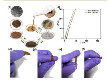
Fig. 3 (a) Schematic of the preparation of thin, flexible OH<sup>-</sup> ion conducting membrane; (b) comparison of Nyquist plots for 3\_OH@PVA at various temperatures and 95% humidity; (c-f) digital photograph of the synthesized membrane and their flexibility at different bending modes.
