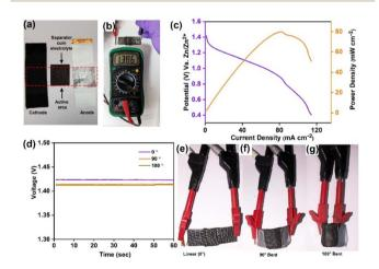
Fig. 5 (a) Components of F-RZABs showing cathode, anode and electrolyte; (b) digital photograph of F-RZAB and multimeter device respectively; (c) recording of the current (I)-voltage (V) polarization plot for F-RZAB; (d) comparative OCV acquired at different bending angles, illustrating the device flexibility; (e-g) digital photograph of the flexible device at various angles (0°, 90°, and 180°).
