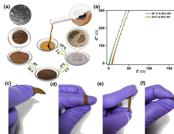
Fig. 3 (a) Schematic of the preparation of thin, flexible OH<sup>-</sup> ion conducting membrane; (b) comparison of Nyquist plots for **3\_OH@PVA** at various temperatures and 95% humidity; (c-f) digital photograph of the synthesized membrane and their flexibility at different bending modes.
