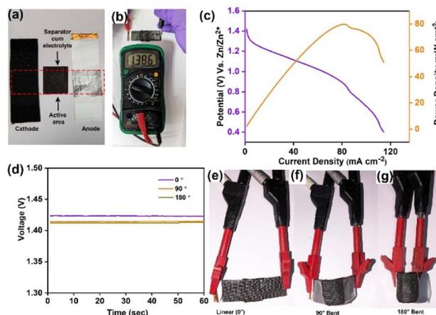
Fig. 5 (a) Components of F-RZABs showing cathode, anode and electrolyte; (b) digital photograph of F-RZAB and multimeter device respectively; (c) recording of the current ( $I$ )–voltage ( $V$ ) polarization plot for F-RZAB; (d) comparative OCV acquired at different bending angles, illustrating the device flexibility; (e–g) digital photograph of the flexible device at various angles ( $0^\circ$ ,  $90^\circ$ , and  $180^\circ$ ).
