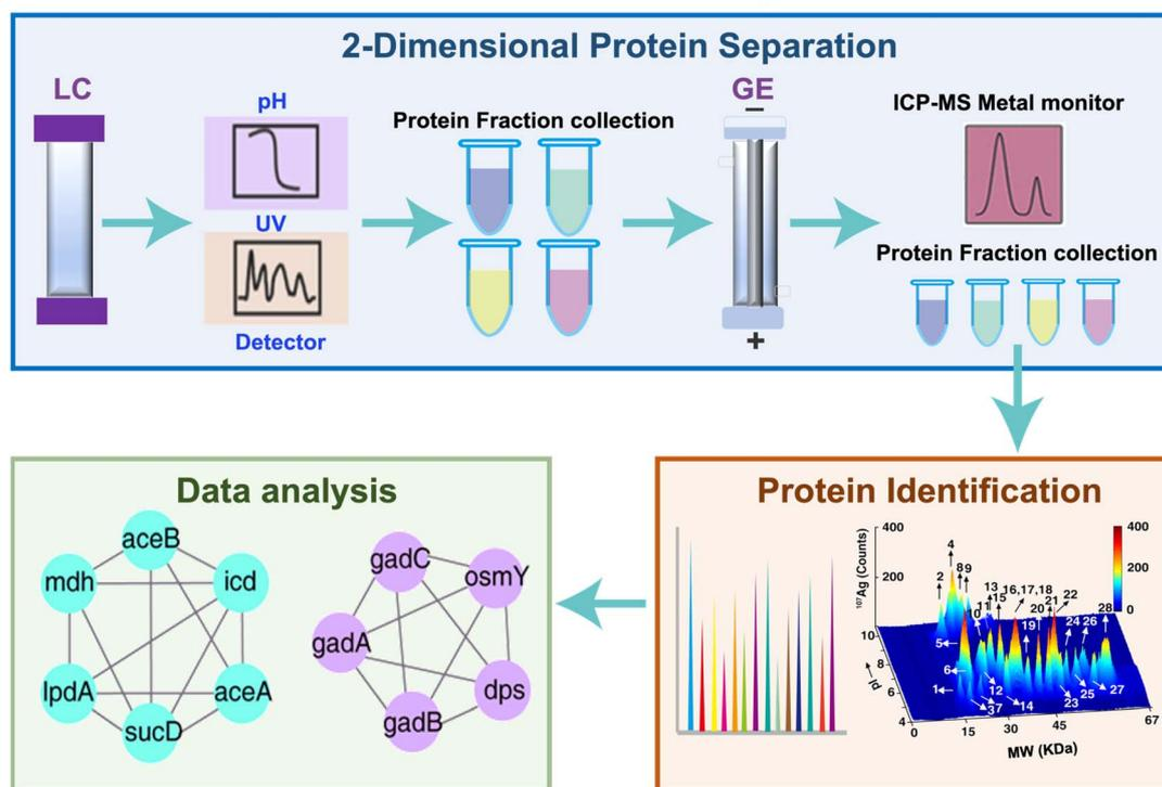
Fig. 2 ICP-MS-based approaches for *in situ* metallome imaging and metalloproteome identification. (A) Characterization of the metallomic profile in tissue sites.<sup>33</sup> (B) General scheme of GE-ICP-MS for tracking metalloproteins.
