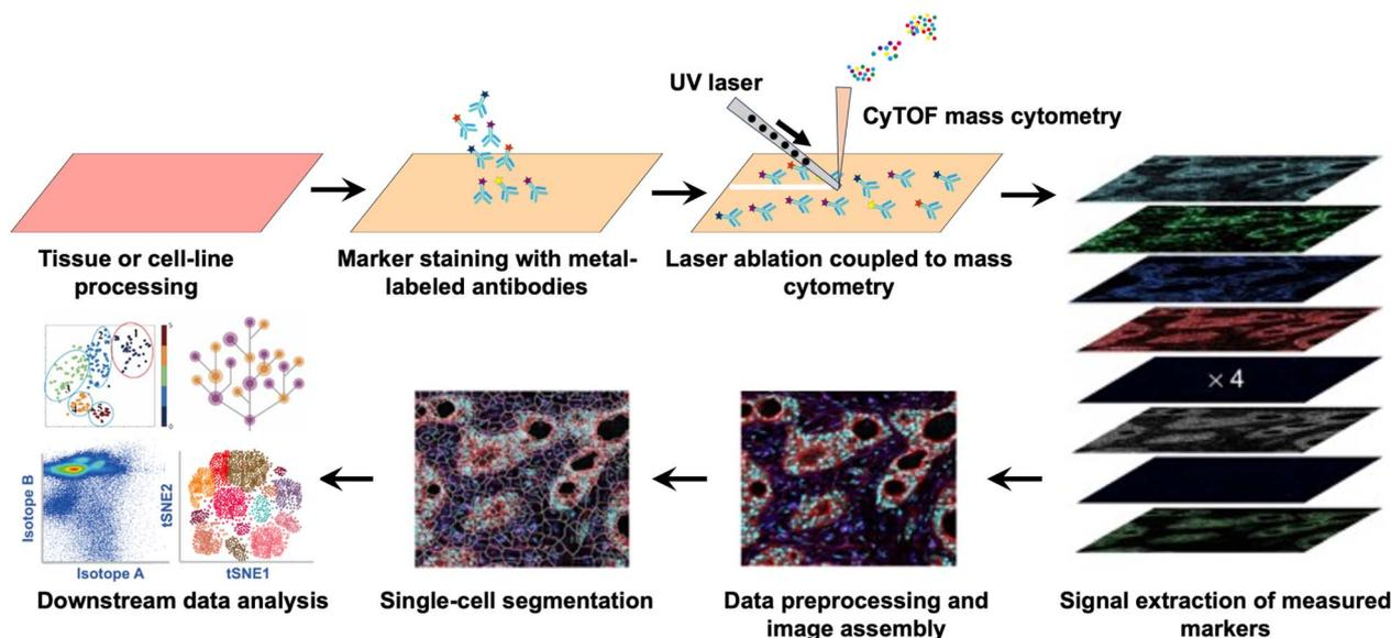
Fig. 4 Workflow of imaging mass cytometry: highly multiplexed imaging of tumor tissues with subcellular resolution by mass cytometry.<sup>42</sup>
