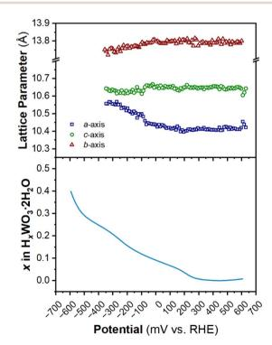
Fig. 11 Trend of lattice parameters (from Pawley refinements of the operando XRD) and proton composition in  $H_xWO_3 \cdot 2H_2O$  (from Fig. 5e) as a function of potential during the cathodic cyclic voltammetry scan in 0.5 M  $H_2SO_4$  at 10 mV  $s^{-1}$ .
