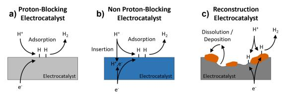
Fig. 1 Schematic representation of three types of electrocatalysts for the HER: (a) proton-blocking electrocatalyst, (b) non proton-blocking electrocatalyst, and (c) reconstruction electrocatalyst.
