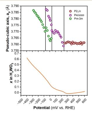
Fig. 7 Pseudo-cubic parameter a (from operando XRD), and proton composition of WO<sub>3</sub> (from Fig. 5b) as a function of potential during a cathodic cyclic voltammetry scan in 0.5 M  $H_2SO_4$  at 1 mV s<sup>-1</sup>.
