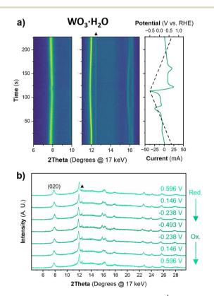
Fig. 8 (a) Operando XRD for  $WO_3 \cdot H_2O$  at 10 mV s<sup>-1</sup> in 0.5 M  $H_2SO_4$ . (b) 1D diffraction patterns showing the full  $2\theta$  region collected and used for Pawley refinements of the structure before and after redox features in the CV. The direction of the CV scan for the 1D diffraction patterns is marked by reduction (Red.) or oxidation (Ox.). The diffraction peak associated with the carbon paper substrate is marked with a triangle.
