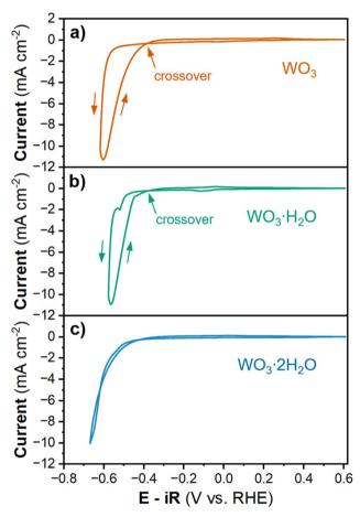
Fig. 3 Cyclic voltammograms of (a) WO $_3$ , (b) WO $_3$ ·H $_2$ O, and (c) WO $_3$ ·2H $_2$ O where the cathodic potential limit was set to the potential where current reaches 10 mA cm $^{-2}$ . The scan rate was 10 mV s $^{-1}$  and rotation rate was 1600 rpm.
