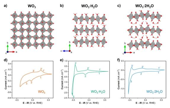
Fig. 2 Crystal structures of (a) monoclinic WO $_3$ , (b) orthorhombic WO $_3$ ·H $_2$ O, and (c) monoclinic WO $_3$ ·2H $_2$ O.  $^{51}$  Cyclic voltammograms of (d) WO $_3$ , (e) WO $_3$ ·H $_2$ O, and (f) WO $_3$ ·2H $_2$ O with a rotation rate of 1600 rpm and scan rate of 10 mV s $^{-1}$  in 0.5 M H $_2$ SO $_4$ .
