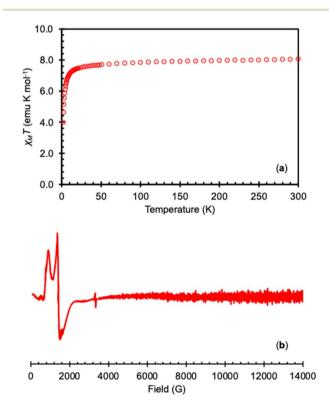
Fig. 3 (a) Plot of  $\chi_{\rm M}T$  versus temperature for isolated 3-Tb<sup>Ph</sup> under an applied field of 1 T and (b) the X-band (9.4 GHz) EPR spectrum of complex 3-Tb<sup>Ph</sup> in toluene (20 mM) at 6 K (bottom).
