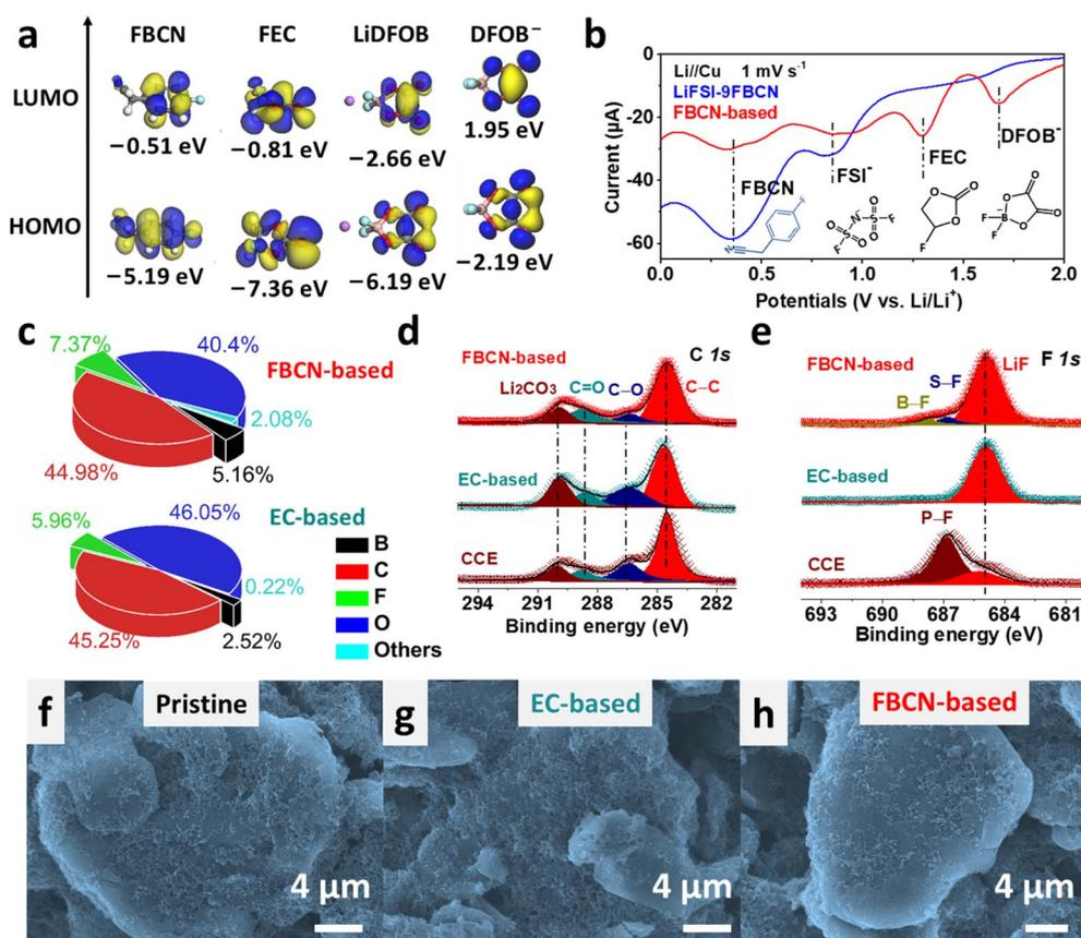
Fig. 4 (a) LUMO and HOMO energy levels for different components. (b) LSV results at  $1$  mV s<sup>-1</sup>. (c) Elemental contents for graphite cycled in various electrolytes. (d) C and (e) F spectra recorded at the graphite surface. SEM images of (f) pristine graphite and graphite cycled in (g) EC-based electrolyte and (h) FBCN-based electrolyte.
