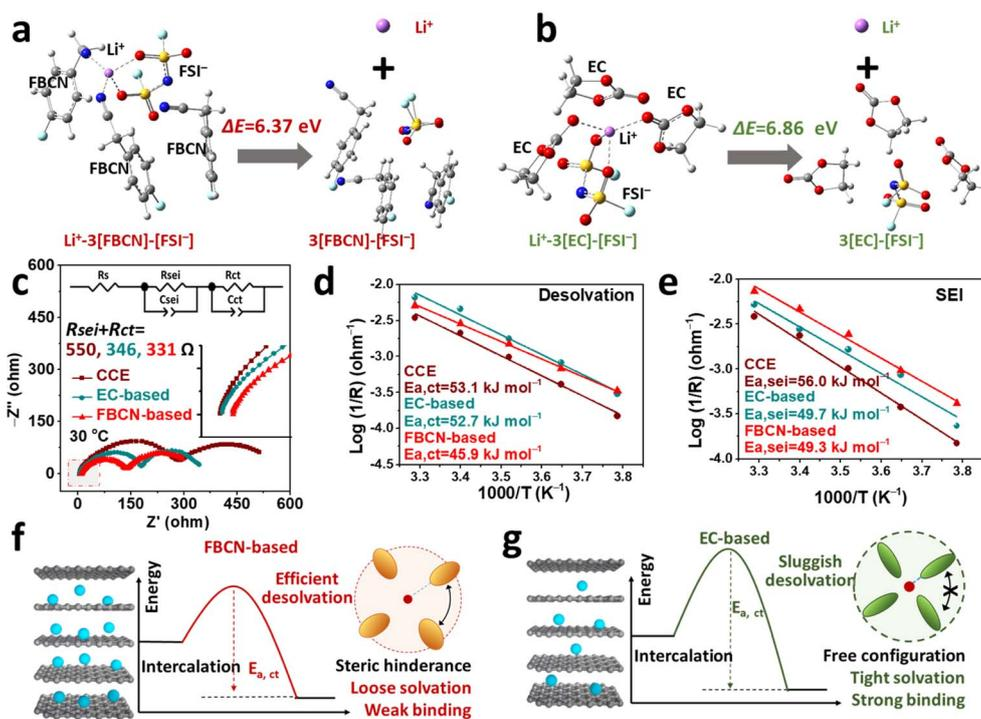
Fig. 5 Energies for removing Li<sup>+</sup> from (a) FBCN-dominated solvates and (b) EC-dominated solvates. (c) EIS results and fitting curves for graphite/graphite cells in various electrolytes. Calculated activation energies for (d) desolvation and (e) Li<sup>+</sup> transport across the SEI in various electrolytes. Illustrations of regulated solvation structures and desolvation in (f) FBCN-based and (g) EC-based electrolytes.
