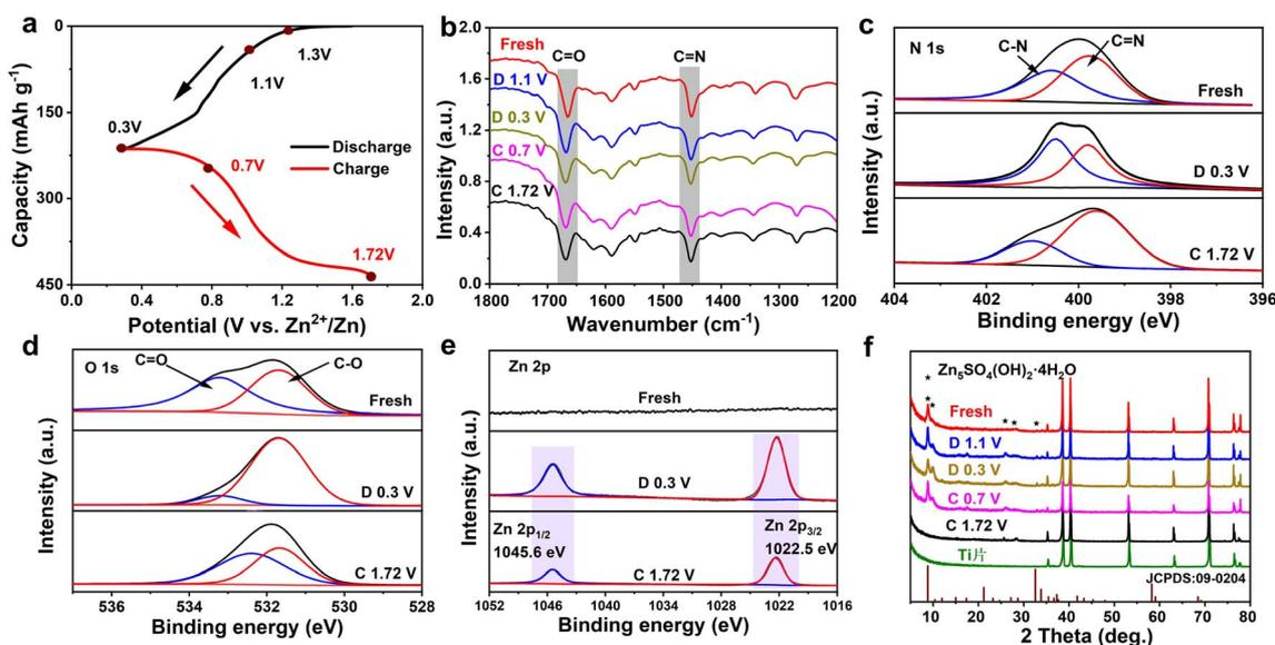
Fig. 5 (a) Charge and discharge profiles of TA-PTO-COF at a current density of  $0.1 \text{ A g}^{-1}$ . (b) *Ex situ* FT-IR spectra of the TA-PTO-COF cathode at different potentials. *Ex situ* XPS analysis of (c) N 1s, (d) O 1s, and (e) Zn 2p. (f) *Ex situ* XRD patterns of the TA-PTO-COF cathode at different potentials.
