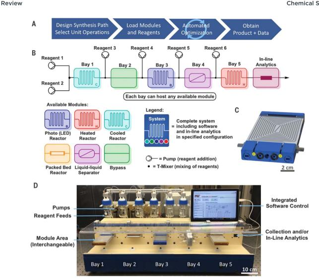
Fig. 10 Plug-and-play, reconfigurable, continuous-flow chemical synthesis system. The workflow (A), the design of the flow system (B) and its actual setup (C) with interchangeable modules (D) are shown in the figure. Reproduced with permission from ref. 115 Copyright 2018, AAAS.
