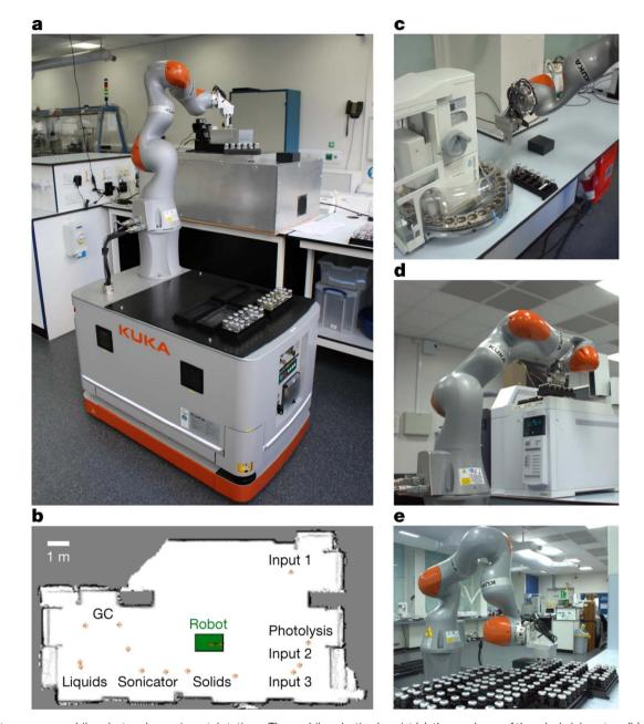
Fig. 6 Autonomous mobile robot and experimental stations. The mobile robotic chemist (a), the roadmap of the whole laboratory (b) and several workstations (c-e) are shown. Reproduced with permission from ref. 4 Copyright 2020, Springer Nature.
