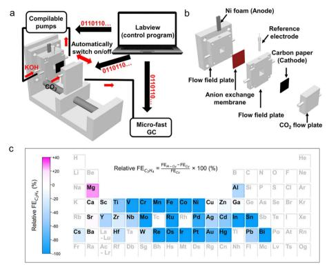
Fig. 9 Fast screening platform for screening bimetallic catalysts for the  $CO_2RR$ . (a) Schematic illustration of the fast screening platform for the  $CO_2RR$ . (b) Exploded view of a 3D-printed flow cell. (c) Heat map of the relative FE of  $C_2H_4$  over Cu-based bimetallic catalysts. Elements in black font represent tested metal salt additives and elements in grey font represent the untested ones. Reproduced with permission from ref. 106 Copyright 2022, Wiley.
