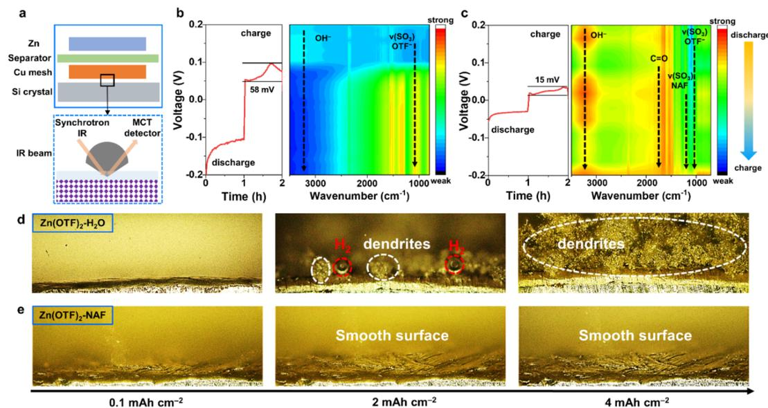
Fig. 3 (a) Schematic diagram of *in situ* ATR-FTIR analysis. (b and c) Voltage–time curves and corresponding ATR-FTIR characterizations in  $\text{Zn}(\text{OTF})_2\text{-H}_2\text{O}$  and  $\text{Zn}(\text{OTF})_2\text{-NAF}$  electrolytes. *In situ* DOF microscope plating images in (d)  $\text{Zn}(\text{OTF})_2\text{-H}_2\text{O}$  and (e)  $\text{Zn}(\text{OTF})_2\text{-NAF}$  electrolytes.
