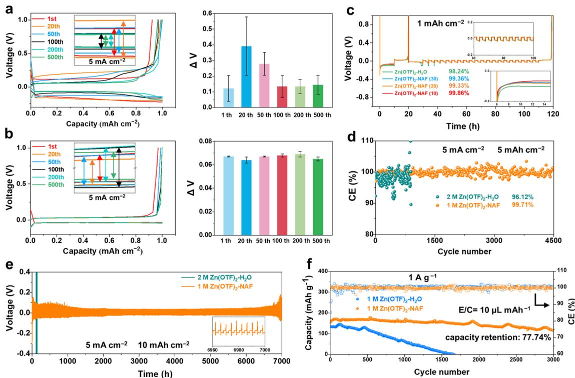
Fig. 5 Long-term deposition voltage–capacity curves and corresponding voltage fluctuation of Zn||Cu cells in (a) Zn(OTF)<sub>2</sub>-H<sub>2</sub>O and (b) Zn(OTF)<sub>2</sub>-NAF electrolytes. (c) Zn||Cu cells with different electrolytes. (d) The plating/stripping CE of Zn||Cu cells. (e) Long-term performance of Zn||Zn cells. (f) Cycling performance of Zn||MnO<sub>2</sub> cells in different electrolytes at 30 °C.
