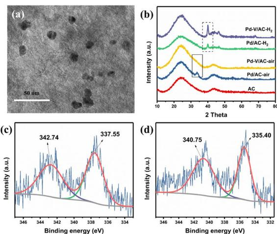
Fig. 1 (a) TEM image of the Pd-V/AC-air catalyst. (b) XRD patterns of various Pd heterogeneous catalysts. (c) XPS spectra of Pd for the Pd-V/AC-air catalyst. (d) XPS spectra of Pd for the Pd-V/AC-H<sub>2</sub> catalyst.
