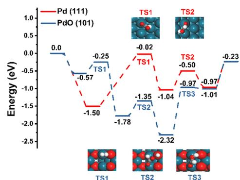
Fig. 3 Potential energy profiles for the hydrogenation of CO<sub>2</sub> to FA on the PdO (101) slab and Pd (111) slab. Structures of transition states are shown in insets. Blue: Pd; red: O; grey: C; white: H.
