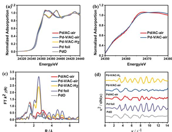
Fig. 2 (a) Normalized Pd K-edge XANES spectra of Pd/AC-air, Pd-V/AC-air, Pd-V/AC-H<sub>2</sub>, Pd foil and PdO. (b) Extended spectra of normalized Pd K-edge XANES spectra of Pd/AC-air and Pd-V/AC-air. (c) Fourier transform of k<sup>2</sup>-weighted EXAFS spectra and (d) EXAFS oscillations of Pd/AC-air, Pd-V/AC-air, Pd-V/AC-H<sub>2</sub>, Pd foil and PdO at the Pd K-edge.
