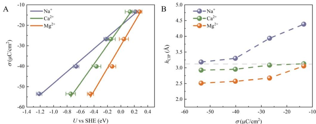
Fig. 2 (A) Plot of surface charge density ( $\sigma$ ) as a function of computed electrode potential ( $U$ ) for the three systems. Surface charge densities scale linearly with computed electrode potential and the slopes indicate the Helmholtz capacitances. (B) Plot of the height of CIP ( $h_{\text{CIP}}$ ) as a function of surface charge density ( $\sigma$ ) for the three systems. The gray dashed line represents the height of the sharp peak in the water density profiles.
