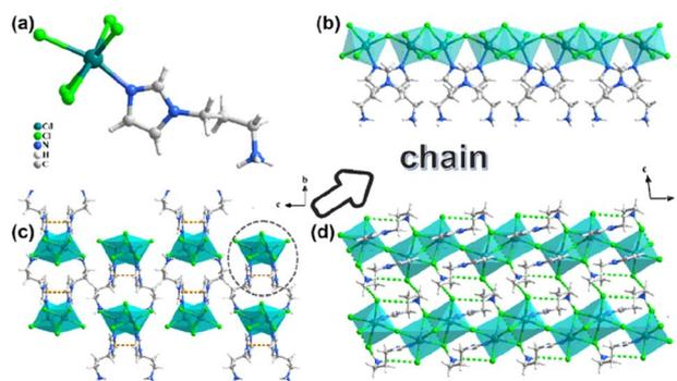
Fig. 1 (a) The asymmetric unit of CdCl-apim1; (b) 1D chain; 3D supramolecular structure along the *a* axis (c) and *b* axis (d) (orange dashed lines:  $\pi \cdots \pi$  interactions; Green dashed lines: N-H $\cdots$ Cl).
