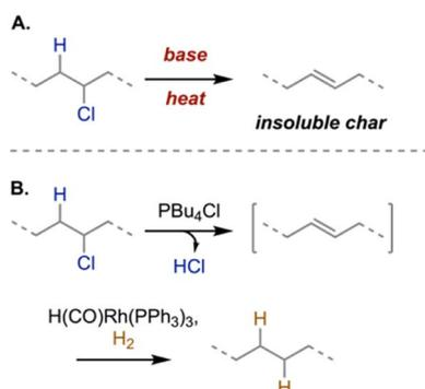
Scheme 5 (A) Dehydrochlorination of PVC *via* elimination leading to insoluble char. (B) Tandem ionic liquid-mediated PVC dehydrochlorination with Rh-catalyzed hydrogenation to form highly saturated but non-linear soluble polymers.<sup>132</sup>
