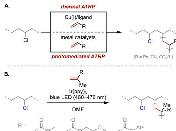
Scheme 4 (A) Thermal and photomediated ATRP for PVC functionalization. (B) An Ir-catalyzed example for generating graft copolymers.<sup>106</sup>
