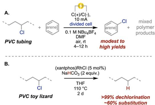
Scheme 6 (A) PVC as a chlorine source for organic synthesis using electrochemistry.<sup>118</sup> (B) Reductive hydrodechlorination using a metal catalyst and a hydride source.<sup>66</sup>
