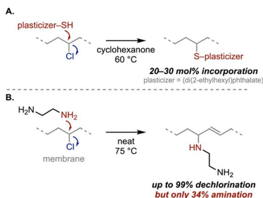
Scheme 2 Nucleophilic substitution reactions on PVC. (A) Covalent incorporation of plasticizer *via* substitution.<sup>63</sup> (B) Competing substitution and elimination observed when PVC is reacted with ethylenediamine.<sup>65</sup>
