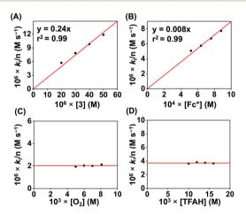
Fig. 10 (A) A plot of  $k_i$  vs. [3] at a fixed concentration of  $O_2$  (8.1 mM), TFAH (20 mM), and Fc\* (1 mM). (B) A plot of  $k_i$  vs. [Fc\*] at a fixed concentration of 3 (0.02 mM), TFAH (20 mM), and  $O_2$  (8.1 mM). (C) A plot of  $k_i$  vs.  $O_2$  at a fixed concentration of 3 (0.02 mM), TFAH (20 mM), and Fc\* (1 mM). (D) A plot of  $O_2$  vs. [TFAH] at a fixed concentration of 3 (0.02 mM), Fc\* (1 mM), and  $O_2$  (8.1 mM).
