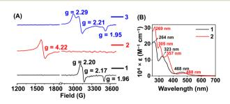
Fig. 1 (A) X-band EPR spectra of 1 (5 mM) and 2 (5 mM) in frozen 9:1 methanol/ethanol at 77 K. The EPR data of 3 (3 mM) were recorded in tetrahydrofuran at 77 K.  $\nu=9.631$  GHz, power = 2.71 mW, modulation frequency = 100 kHz, modulation amplitude = 4.91 G. (B) UV-vis spectra of 1 (0.5 mM) and 2 (0.5 mM) in acetonitrile at 25 °C.
