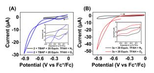
Fig. 7 Cyclic voltammograms of **2** (0.5 mM, (A)) and **3a** (0.5 mM, (B)) in the presence and absence of oxygen in acetonitrile containing 10 mM of TFAH and 50 mM  $^n\text{Bu}_4\text{NPF}_6$  as the supporting electrolyte at 25 °C. The inset data show a zoomed version of the Fe<sup>III</sup>/Fe<sup>II</sup> potential region. CV data were recorded using a 3 mm GC electrode at a 100 mV s<sup>-1</sup> scan rate.
