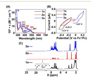
Fig. 3 (A) UV-vis spectra of 1a (0.5 mM), 2a (0.5 mM), and 3a (0.5 mM) in acetonitrile at 25 °C. (B) Cyclic voltammogram of the Fe<sup>II</sup> complexes (0.5 mM) in acetonitrile containing 50 mM of  $^{n}Bu_{4}NPF_{6}$  as the supporting electrolyte at 25 °C (scan rate 5 mV s<sup>-1</sup>), using a 3 mm glassy carbon working electrode and Pt wire counter electrode. (C)  $^{1}H$ -NMR spectrum of the Fe<sup>II</sup> complexes in CD $_{3}$ CN at 25 °C.
